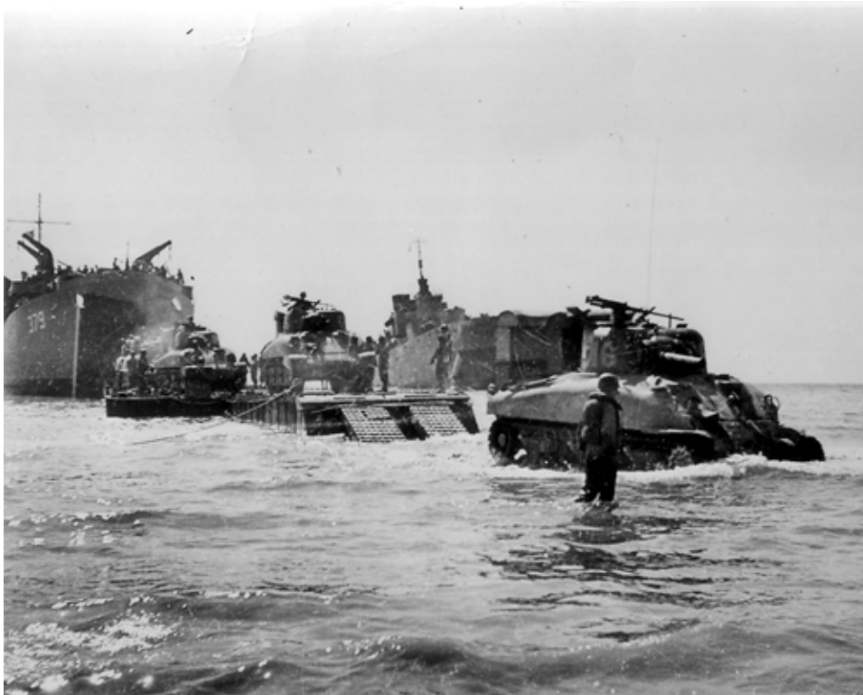
SC-181222: Tanks from the 191st or 751st Tank Battalion debark across a pontoon from an LST at Salerno on 9 September 1943. This method, also used in the Sicily landings, was slow and vulnerable to enemy fire. (Signal Corps photo)
