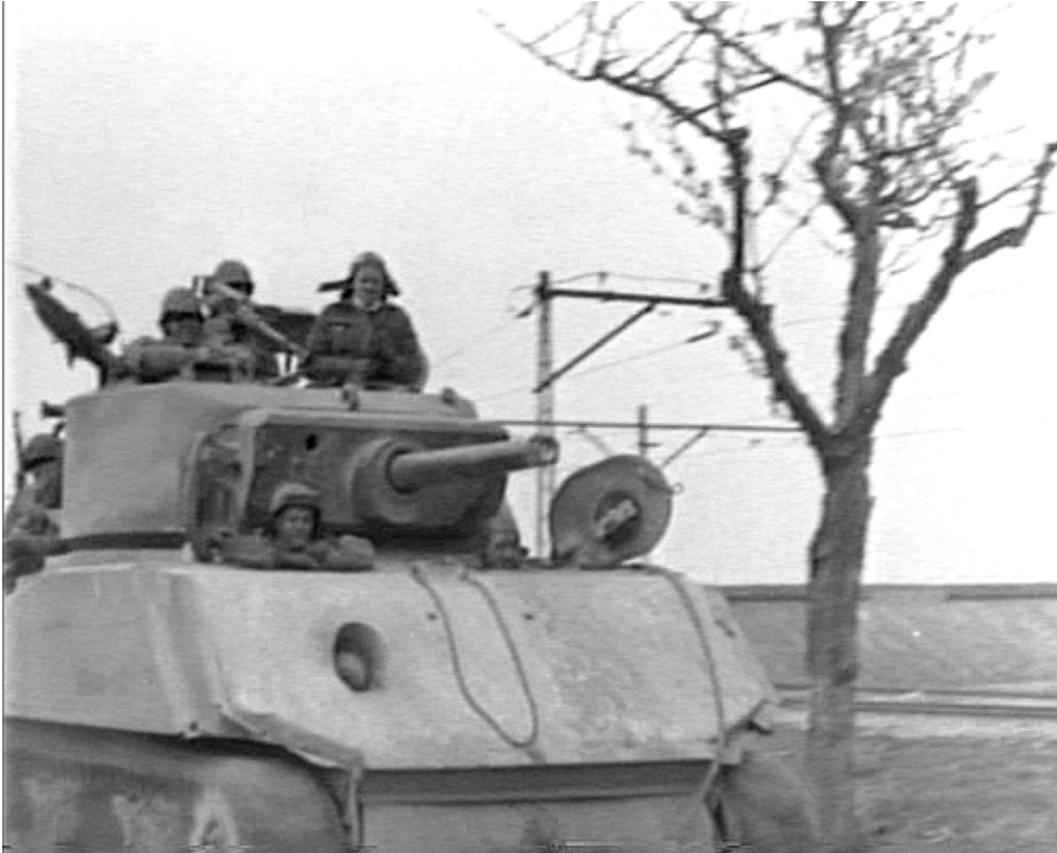
111-ADC-4025_6: The M4A3E2 Jumbo assault Sherman appeared only in the European theater. The 750th Tank Battalion added a layer of concrete to the Tiger-tank-thick front armor on this Jumbo, seen on the road to Halle in April 1945. (Signal Corps film)
