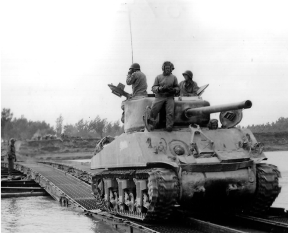
SC-208319: A 757th Tank Battalion M4A3 (76mm) crosses the Po River on 26 April 1945. After soldiering with the oldest tanks in the arsenal into 1944, tankers in Italy caught up with their counterparts in the European theater by early 1945. (Signal Corps photo)
