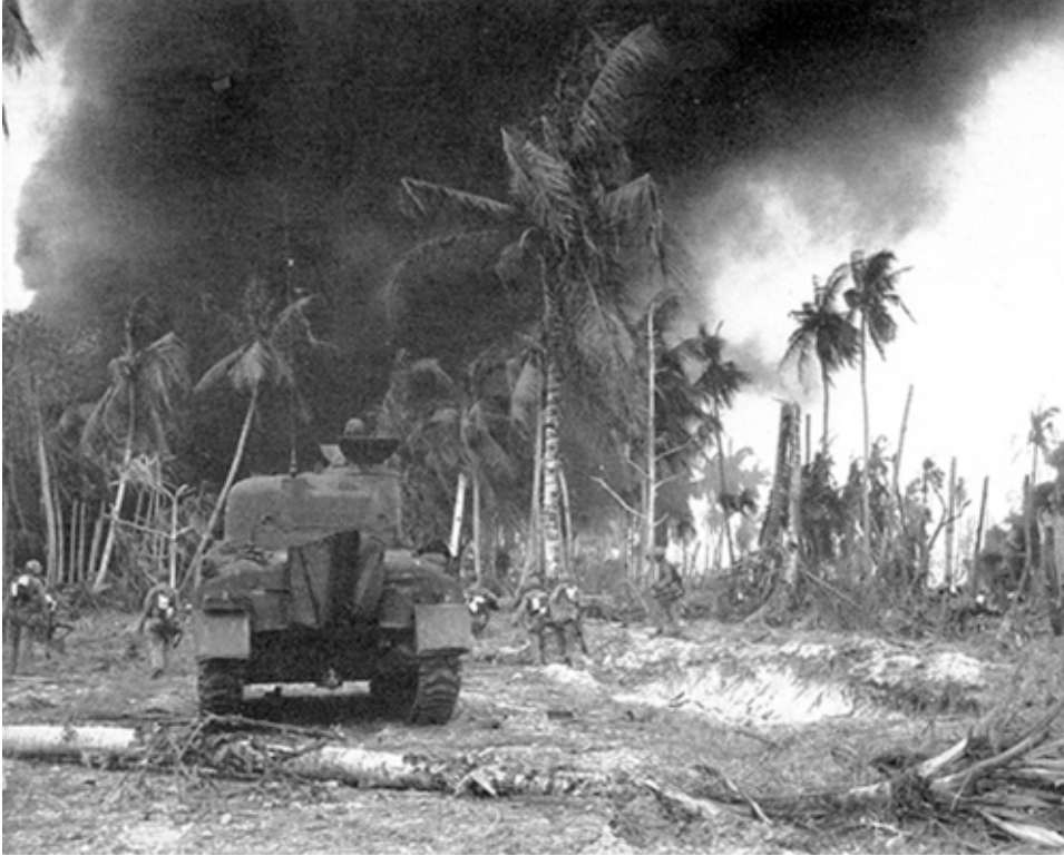
Army 17: A 767th Tank Battalion Sherman works with 7th Infantry Division doughs on Kwajalein in February 1944. A field phone is mounted on the left-rear fender, one of the first experiments in improving tank-infantry communications. (U.S. Army Photo)
