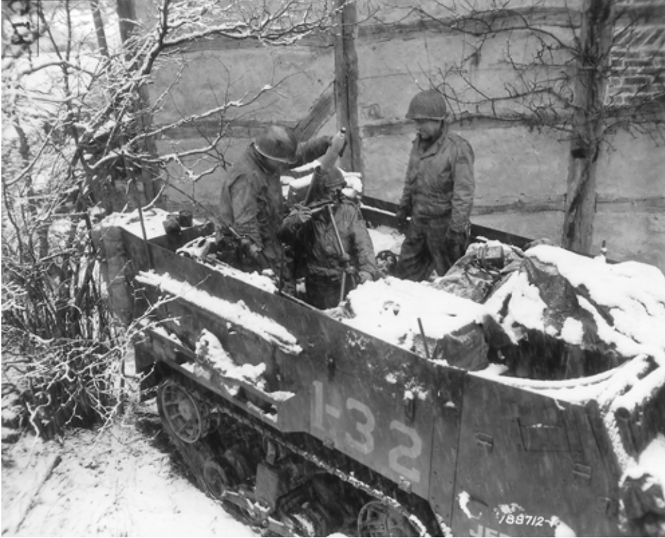
SC-188712: The Mortar Platoon in light, medium, and standard tank battalions used half-track-mounted 81mm mortars such as this M4A1 Mortar Carrier, at work in Belgium in early 1945. Some outfits made good use of the platoon, but many did not. (Signal Corps photo)
