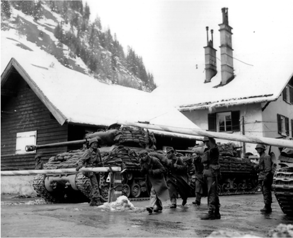
SC-204477-S: 781st Tank Battalion Shermans reach the frontier in Brenner Pass, where Seventh Army linked up with Fifth Army, on 4 May 1945. The Easy 8 (left) was the final stage of the Sherman's development, but tankers still resorted to sandbagging for better armor protection. (Signal Corps photo)
