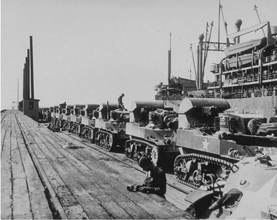
756thTorchSigCorps: M5 light tanks belonging to the 756th Tank Battalion (Light) await loading for the journey to North Africa for Operation Torch. They are waterproofed and fitted with wading stacks much like those that will be used in amphibious landings for the rest of the war. (Signal Corps photo)
