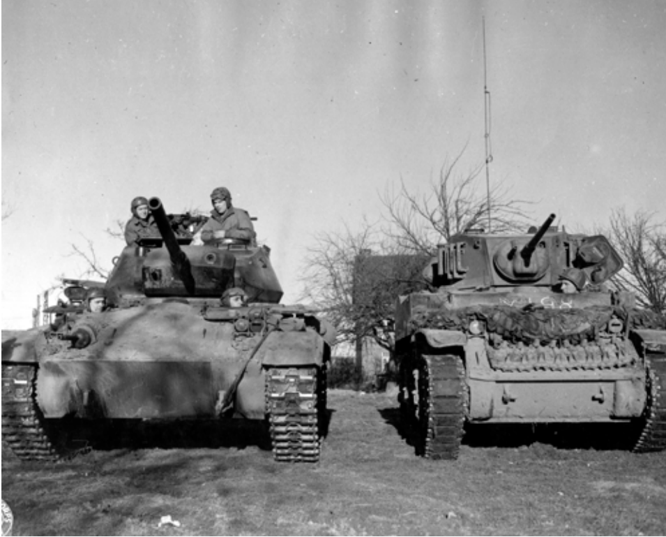
744thM24M5: The M24 Chaffee light tank and the M5 that it replaced, both belonging to the 744th Tank Battalion (Light). The 740th Tank Battalion first used two M24s in battle when it found them at a replacement depot during the Battle of the Bulge. (Signal Corps photo)
