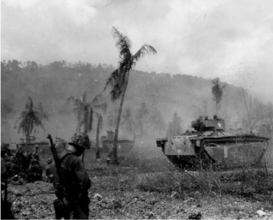
89974: LVT(A)(1) (left) and LVT(A)(4) amtanks belonging to Company D, 708th Amphibian Tank Battalion, line up to attack with the Marines on Saipan in June 1944. (Marine Corps photo.)
