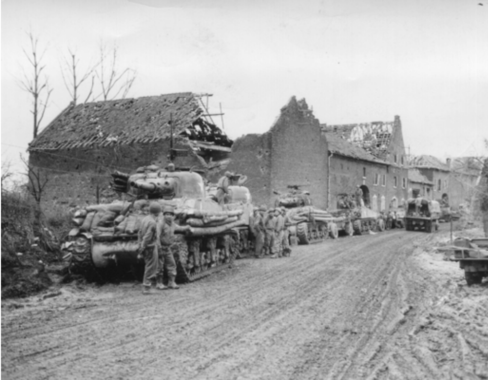
111-SC-197299: Shermans from the 771st Tank Battalion form up before the next attack toward Linnich in 29 November 1944. The tanks carry logs to put under the tracks for traction should a tank bog down in the mud. (National Archives, Signal Corps photo)
