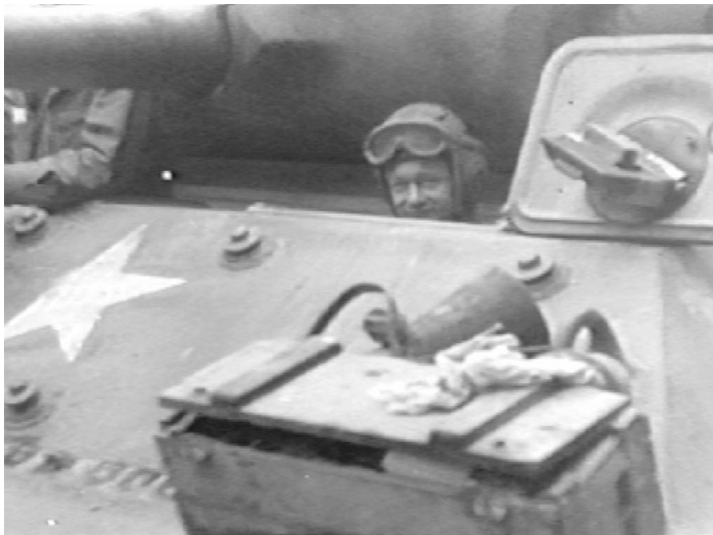
111-ADC-3991_2: The type of periscope used by the driver and assistant driver is visible on the lower surface of the open hatch cover. (National Archives, Signal Corps film)
