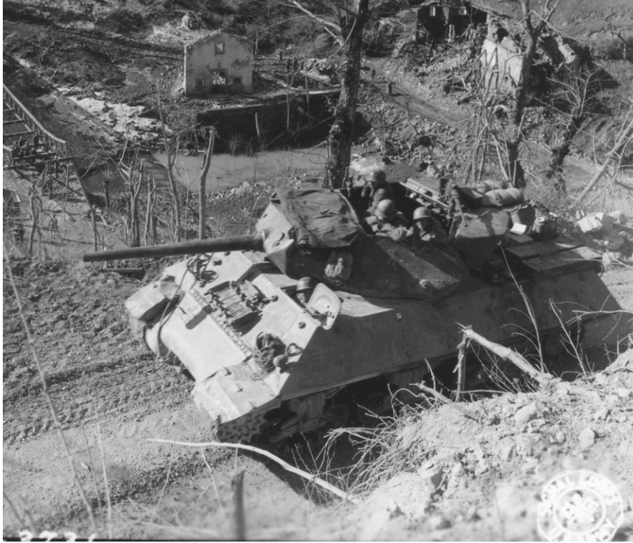
SC-329838: This 701st Tank Destroyer Battalion M10 near M. Terminale, Italy, in March 1945 offers a good look at how exposed the crewmen in the turrets were to enemy fire and the elements. (National Archives, Signal Corps photo)
