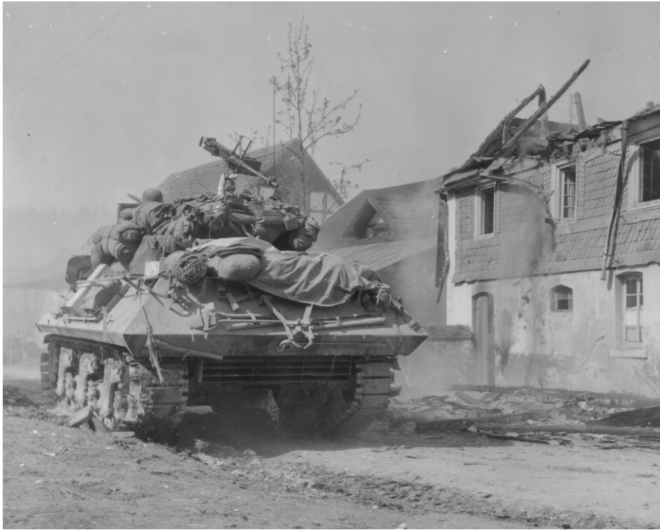
SC-279965: A crewman crouches behind a forward mounted machine gun during fighting to clear Odingen, Germany, in April 1945. Note the grousers on the M10's tracks used to improve mobility in mud and snow; many have snapped off, which was a major weakness of the grousers. (National Archives, Signal Corps photo)
