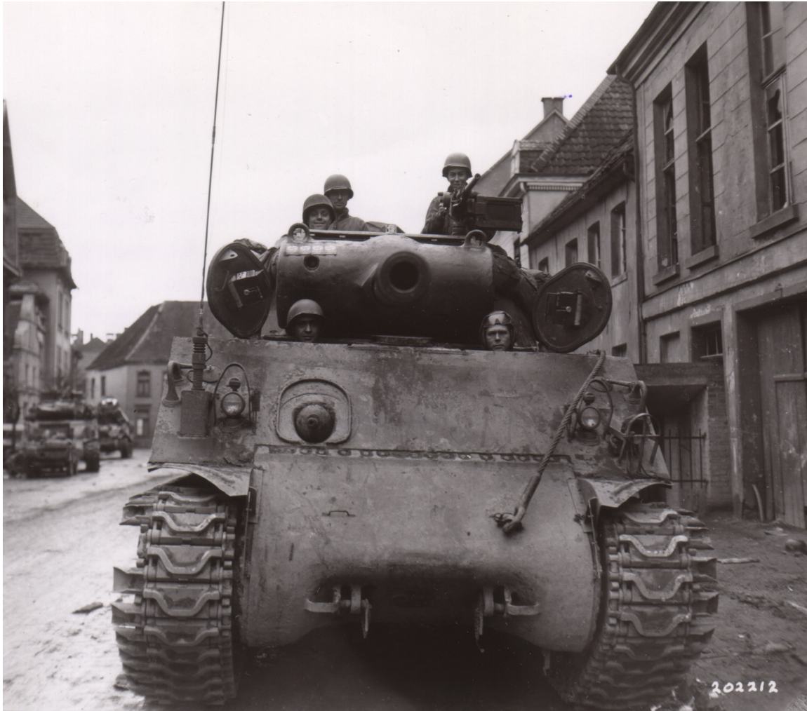
SC-202212: The business end of the rare M36B1—with an M36 turret mounted on a Sherman chassis—in March 1945. In addition to the hull machine gun, the turret .50-caliber has been remounted facing forward. The M36B1 variant all but erased the distinction between a tank and a tank destroyer. This crew had been credited with destroying two Mark IVs and two Tigers. (National Archives, Signal Corps photo)
