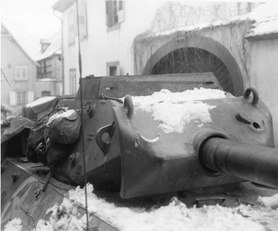
SC-199129: View of the steel turret cover eventually installed by the 813th Tank Destroyer Battalion on its M10s to protect the crews from shrapnel and grenades, January 1945. (National Archives, Signal Corps photo)
