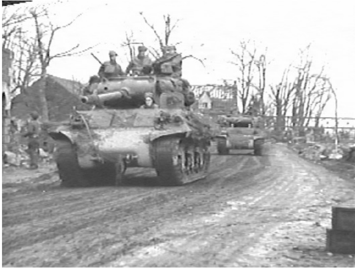
111-ADC-2131_1: The 702d Tank Destroyer Battalion motors to a pontoon bridge to cross the Roer River on 26 February 1945. This M36 has extra armor plates welded onto the glacis in front of the driver and assistant driver positions. (National Archives, Signal Corps film)
