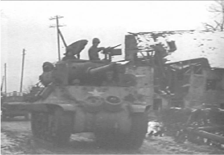
111-HRB-30_11: An M36 passes through a destroyed village during the drive toward the Roer River in late November 1944. The vehicle has an extra machine gun mounted on the turret front for use against ground targets, a field solution that was becoming popular in TD outfits. The anti-aircraft machine gun is covered. (National Archives, Signal Corps film)
