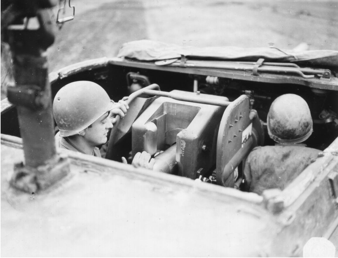
SC-195752: Loading a 90mm round in an M36. (National Archives, Signal Corps photo)
