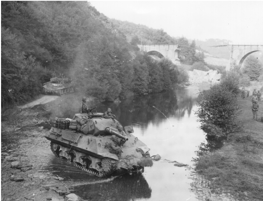
SC-194148: Tank destroyers cross a stream near Hammeras, Germany, in September 1944. Note the hedge cutters mounted on the final drive housing, and that a crewman must ride on the rear deck in order to use the machine gun against ground targets in the direction of main gun. (National Archives, Signal Corps photo)
