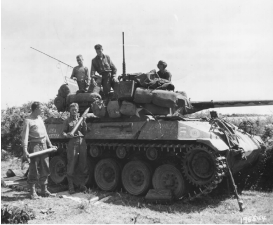
SC-195544: M18 crewmen load 76mm shells outside Brest in August 1944. (National Archives, Signal Corps photo)
