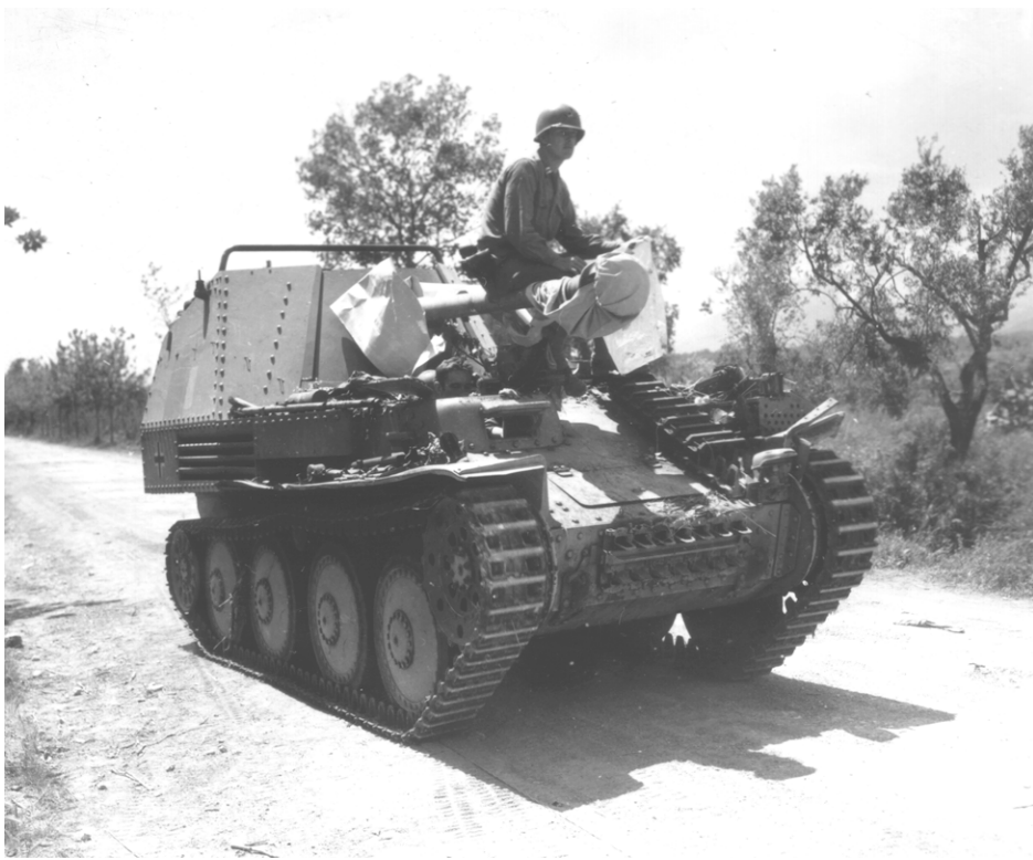
SC-329843: An early model German self-propelled antitank gun, the Marder III, captured in Italy in May 1944. The vehicle carried a 75mm gun on a light tank chassis. (National Archives, Signal Corps photo)
