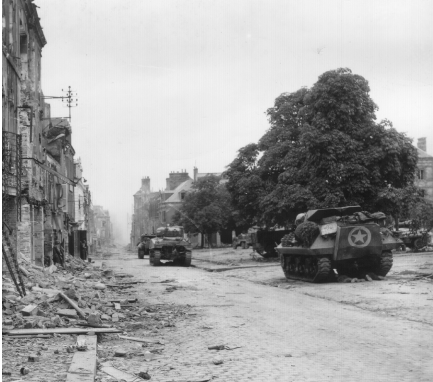
SC-191820: M10s, Shermans, and doughs enter St. Lô in Normandy on 21 July 1944. This photo illustrates the increasingly standard practice of keeping TDs a short distance behind the lead tanks to provide fire support. Note the exhaust stack used to prevent engine flooding during the landings, still attached to the rear of the M10. (National Archives, Signal Corps photo)
