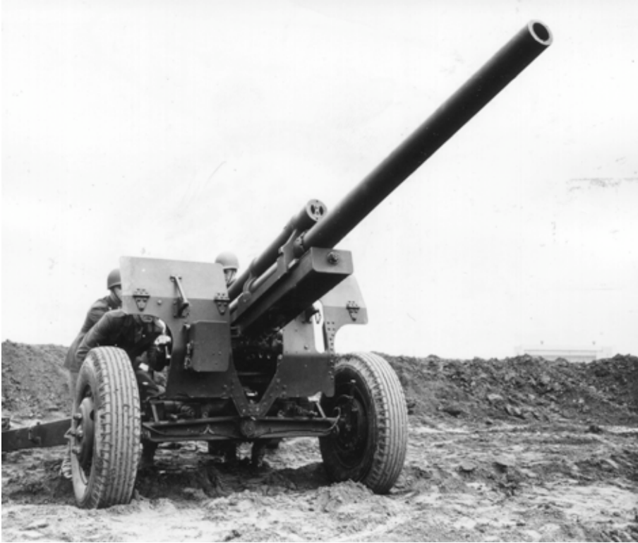
189896: The towed 3" gun undergoing testing at Aberdeen Proving Grounds. The Signal Corps caption observes, "Army Ordnance Department tests have proved the 3" antitank gun as superior to the German 88mm antitank gun as an antitank weapon." Ordnance was wrong. (National Archives, Signal Corps photo)
