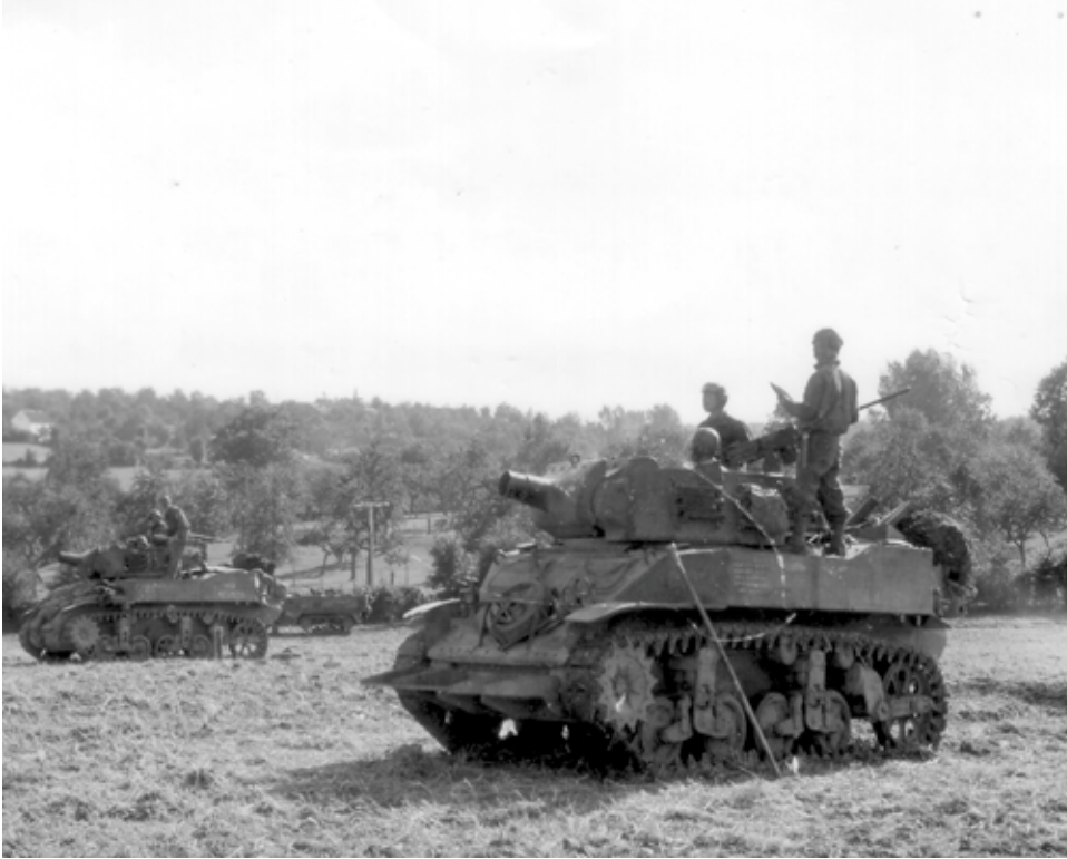
SC-194105: M8 HMC assault guns belonging to the 113th Cavalry Reconnaissance Squadron prepare to fire in Belgium on 9 September 1944, near the end of the "rat race" to the German frontier. The nearest vehicle sports a hedgerow cutter. (Signal Corps photo)
