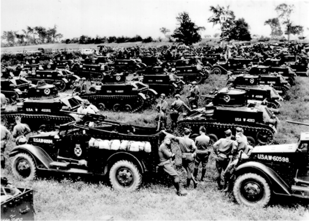
SC-114290: Mechanized cavalry assemble during First Army maneuvers in August 1939 as war looms in Europe. The M3A1 scout cars in the foreground have just entered service, and the M1A1 "combat cars" behind are obsolete. (Signal Corps photo)
