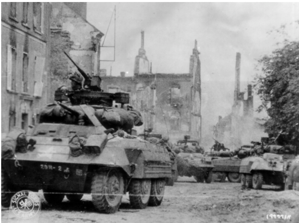
SC-199771: Armored cars belonging to the 29th Cavalry Reconnaissance Troop in the ruins of St. Lo, France, on 20 July 1944. Note the field-expedient .50-caliber anti-aircraft gun. (Signal Corps photo)
