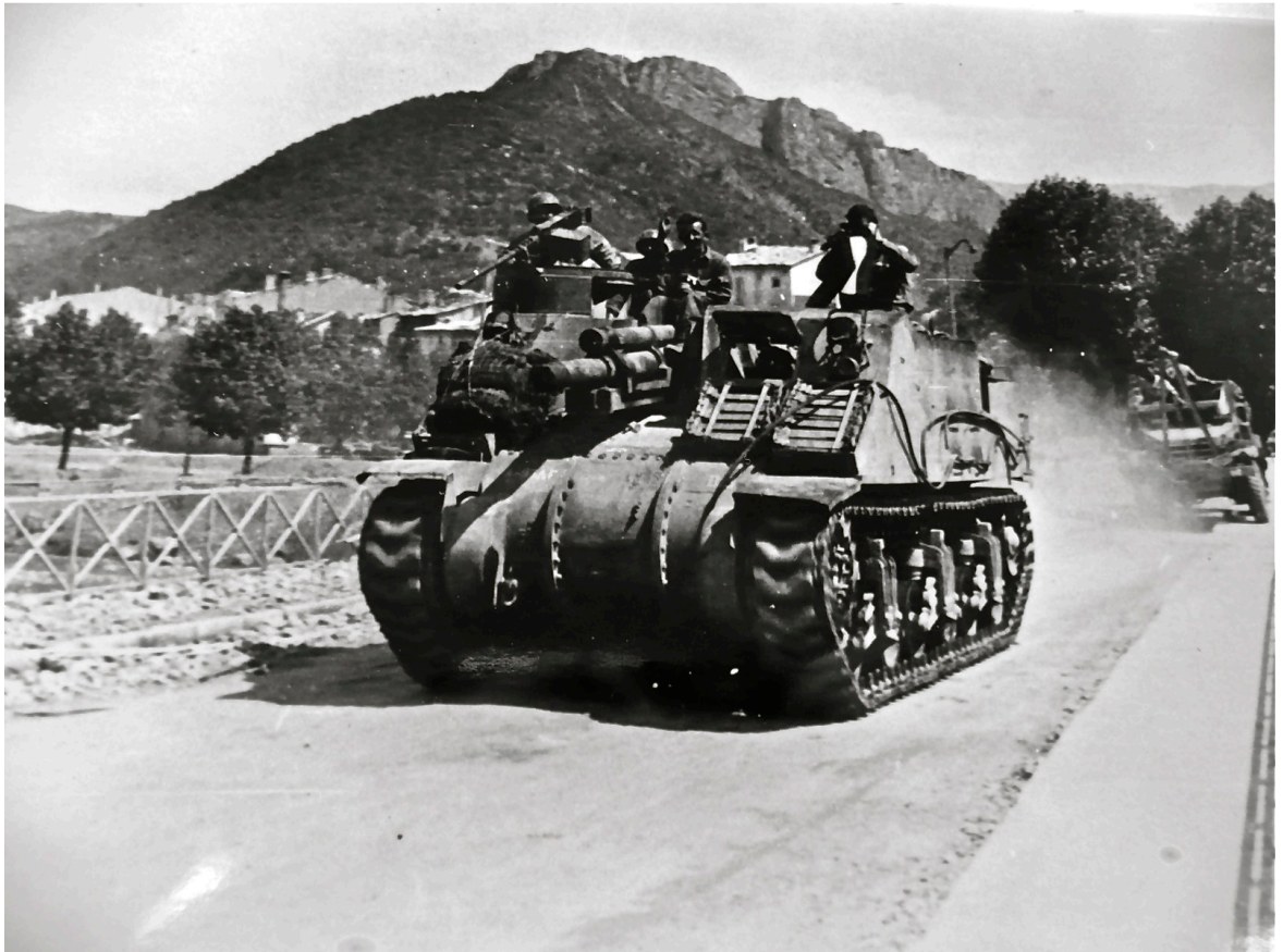
Hodge somehow managed to get an issue of M7 Priest self-propelled 105mm guns for his squadron's assault gun troop. All other cavalry squadrons were equipped with the much less powerful M8 75mm Gun Motor Carriage. This one is pictured in France.
