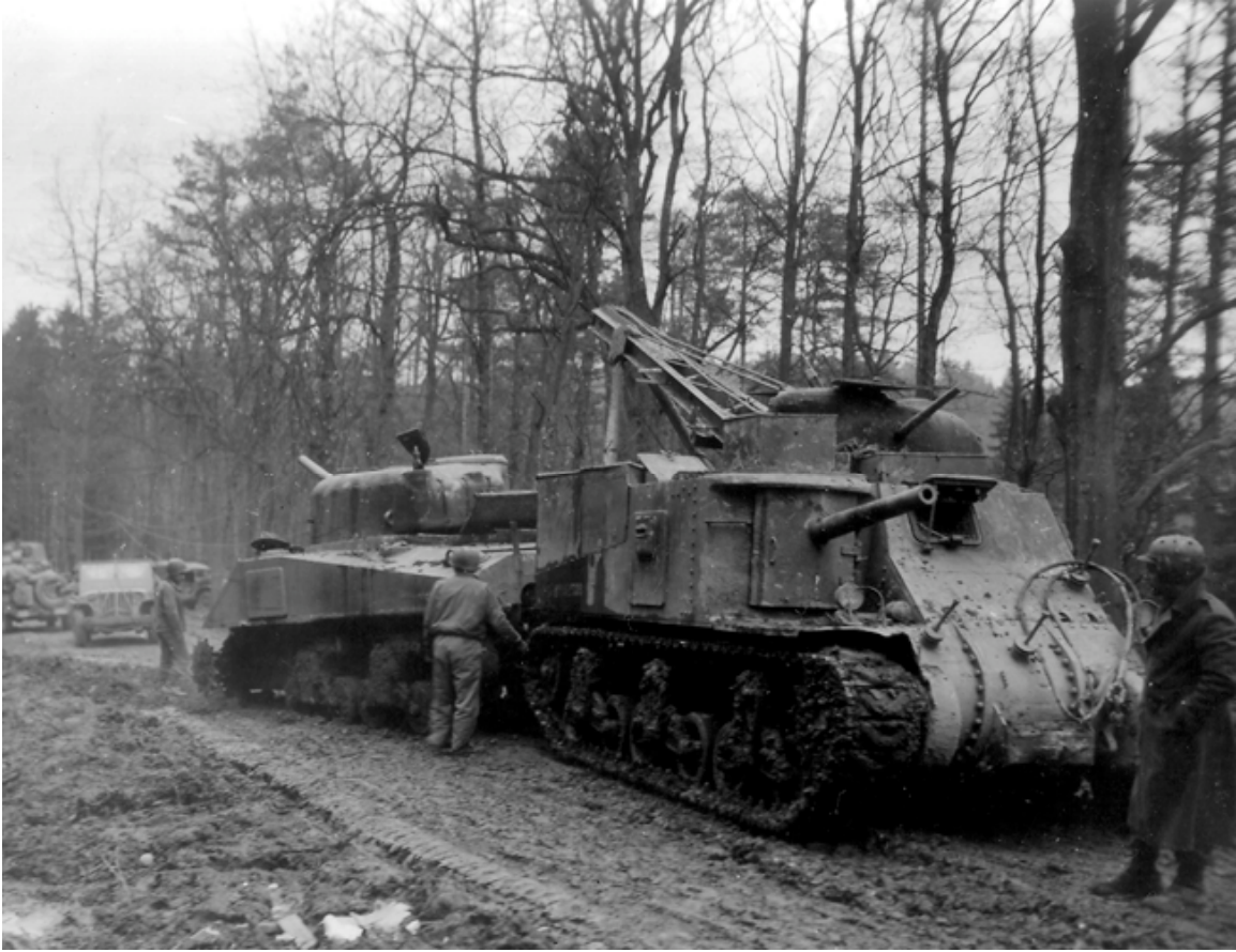
SC-197756: A T2 recovers a Sherman near Grosshau, Germany, in December 1944. Note the handle on the sponson door beside the fake 75mm gun. (NARA, Signal Corps photo)
