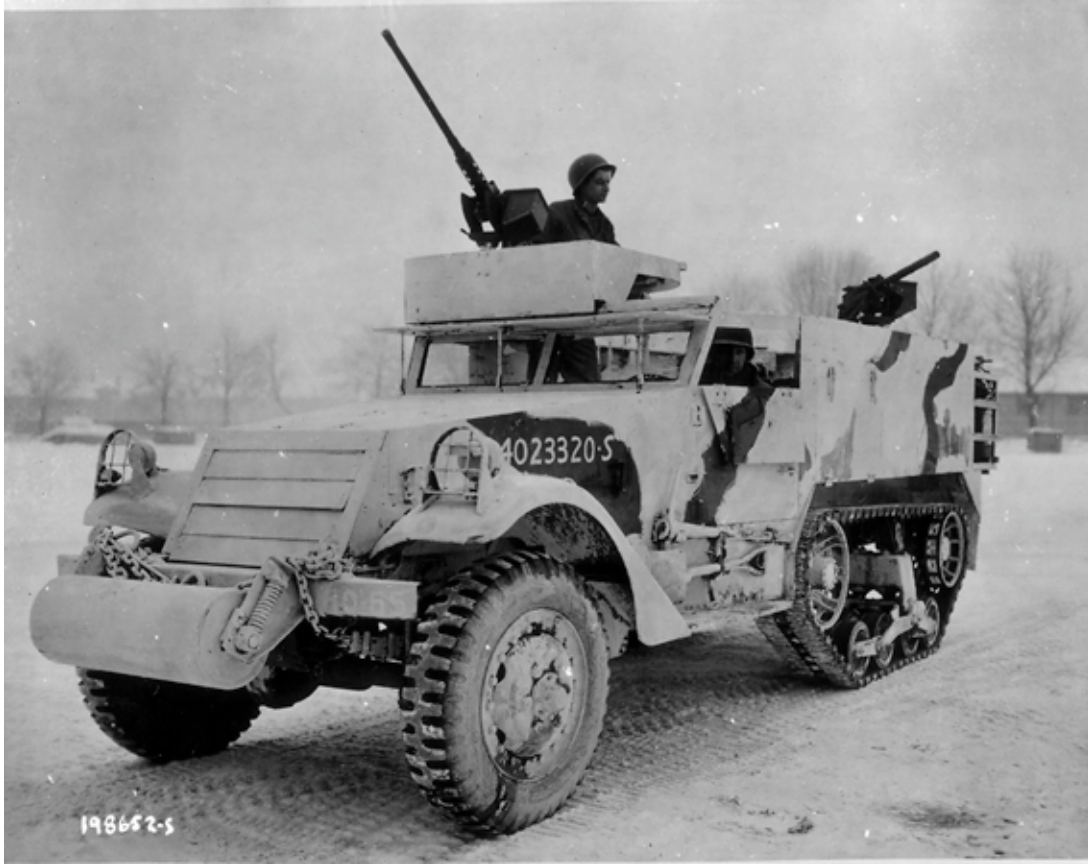
SC-198652-S: M2A1 and M3A1 halftracks added a ring mount for a .50-caliber machine gun. (NARA, Signal Corps photo)
