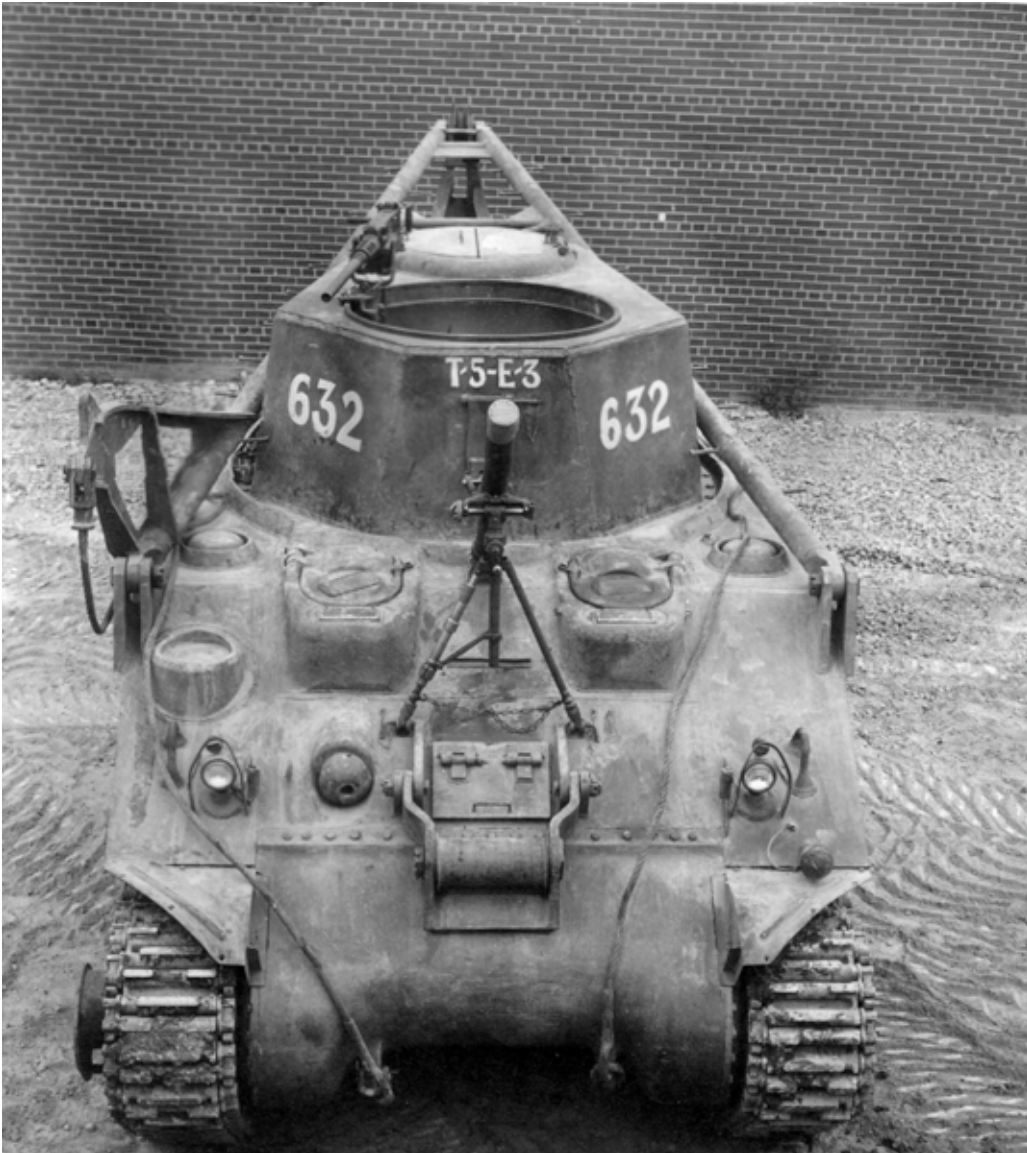
AFB5977: A tank recovery vehicle T5E3 (development vehicle for the M32) displays the 81mm mortar when mounted. (NARA, U.S. Army photo)
