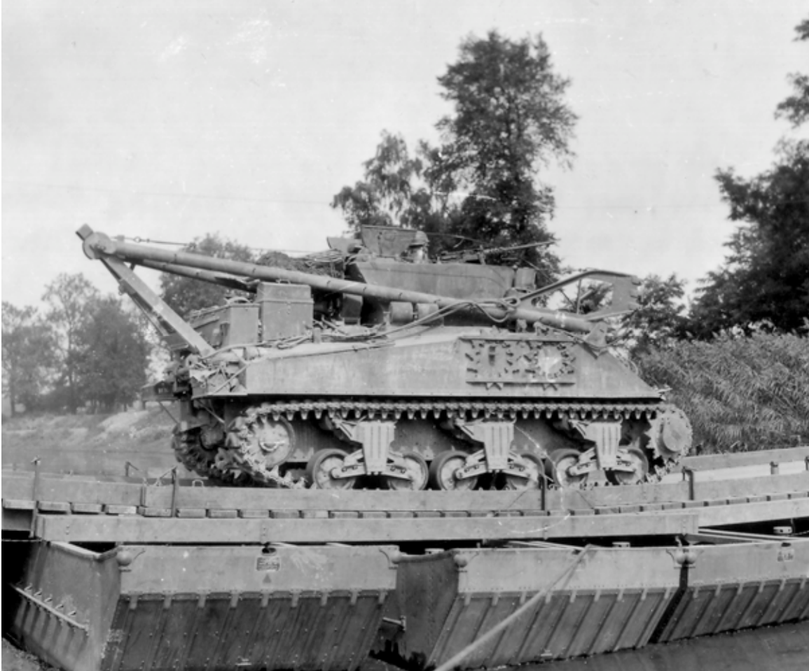
SC-194536: An M32 tank retriever in France in September 1944. (NARA, Signal Corps photo)
