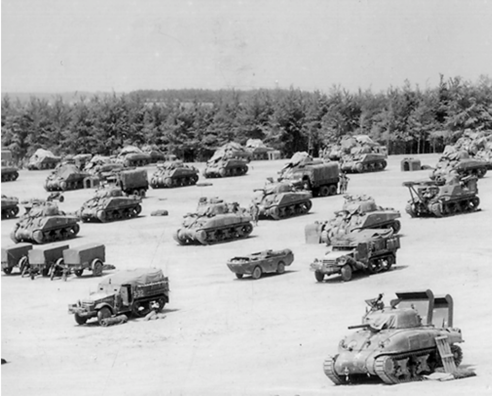
SC-186584: This tank battalion from the 66th Armored Regiment, 2d Armored Division, is gathered at a marshalling area on 29 May 1944. The photo shows tanks with and without wading gear, halftracks, deuce-and-a-half cargo trucks, a T2 tank recovery vehicle, and a non-standard-issue 1/4-ton amphibian truck. (NARA, Signal Corps photo)
