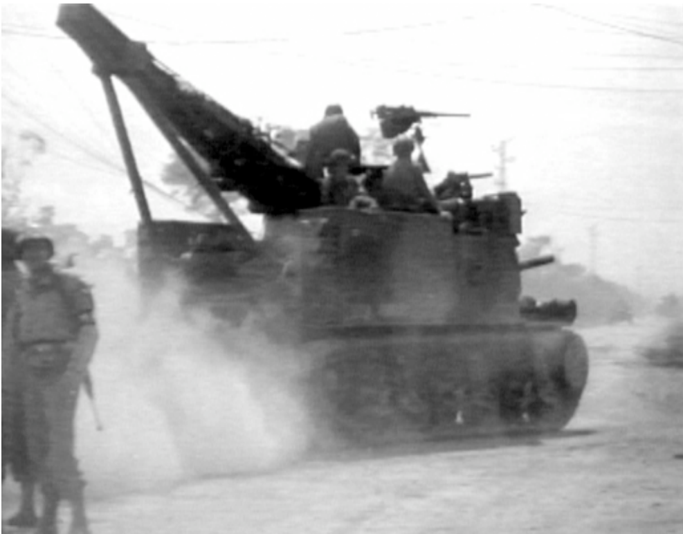
111-ADC-1677_2: A 2d Armored Division T2 advances during Operation Cobra in July 1944. Note the extra .50-caliber machine gun atop the turret and what appears to be a .30-caliber below and to the right of that. (NARA, Signal Corps photo)
