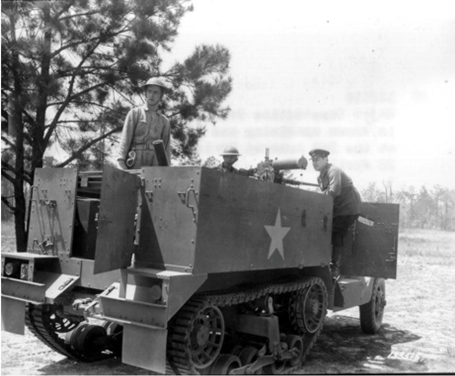
SC-133515: A Soviet officer in April 1942 examines a 2d Armored Division Halftrack 81mm Mortar Carrier M4, based on the M2 halftrack. The shorter rear compartment and twin back steps are the easiest way to distinguish the M2 from the M3 halftrack. (NARA, Signal Corps photo)
