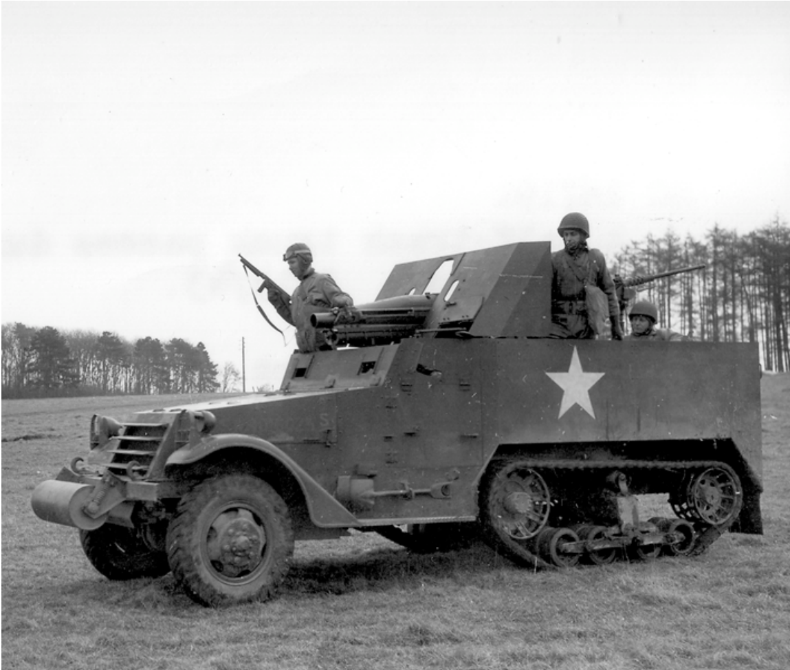
SC-167191: A T30 assault gun displays the distinctive hump atop the 75mm pack howitzer barrel. The pedestal-mounted .50-caliber machine gun is visible behind the howitzer. (NARA, Signal Corps photo)
