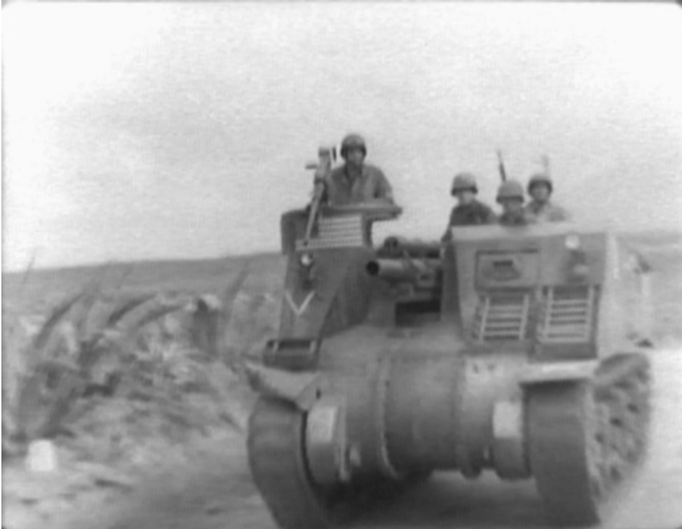
111-FB-51_1: The 1st Armored Division, while still in North Africa in November 1943, assigned M7 Priest self-propelled 105mm howitzers to its medium tank battalions as stop-gap assault guns, because it found the 75mm howitzer underpowered in combat. The 751st substituted M7s for its M8s when it reorganized as a standard tank battalion in December 1943 while in Italy. (NARA, Signal Corps film)
