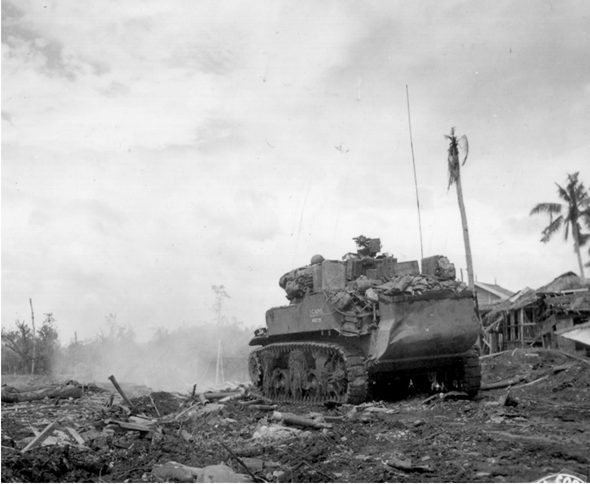
SC-199172: An M8 fires at a Japanese pillbox on Leyte Island, the Philippines, in December 1944. Close-quarters shooting was common in the Pacific Theater. This assault gun still has part of its wading gear attached. (NARA, Signal Corps photo)
