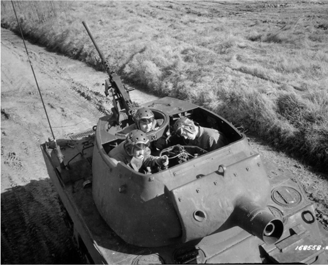
SC-168558-R: Layout of the M8 turret, which was also installed on the LVT(A)(4) amtank. (NARA, Signal Corps photo)
