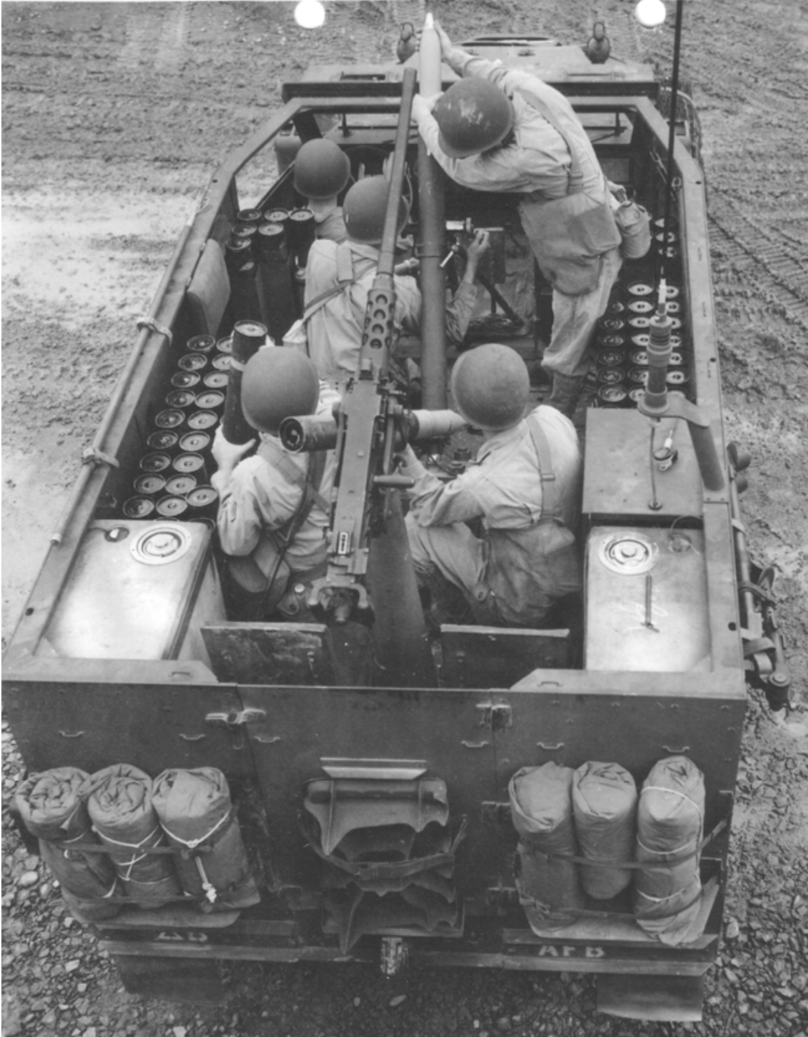
AFB6100: The crew of an 81mm Mortar Carrier T19, prototype for the M21, serves the weapon, which was designed to fire forward. (NARA, records of the Chief of Ordnance)
