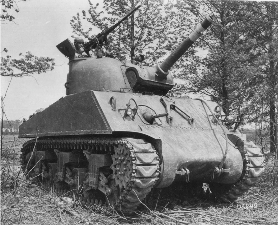
SC-192647: An early M4 Sherman with 105mm howitzer. This vehicle has a standard commander's hatch. (NARA, Signal Corps photo)
