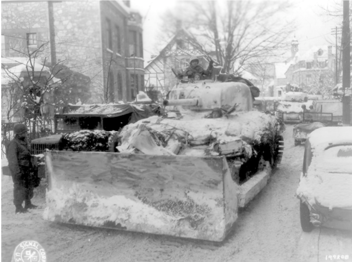
SC-199208: A tank dozer leads an armored column through Malmedy, Belgium, on 13 January 1945 clearing snow where necessary. The tank dozer was not a particularly good plow as deep snow mounded up quickly in front of the straight-on blade. (NARA, Signal Corps photo)
