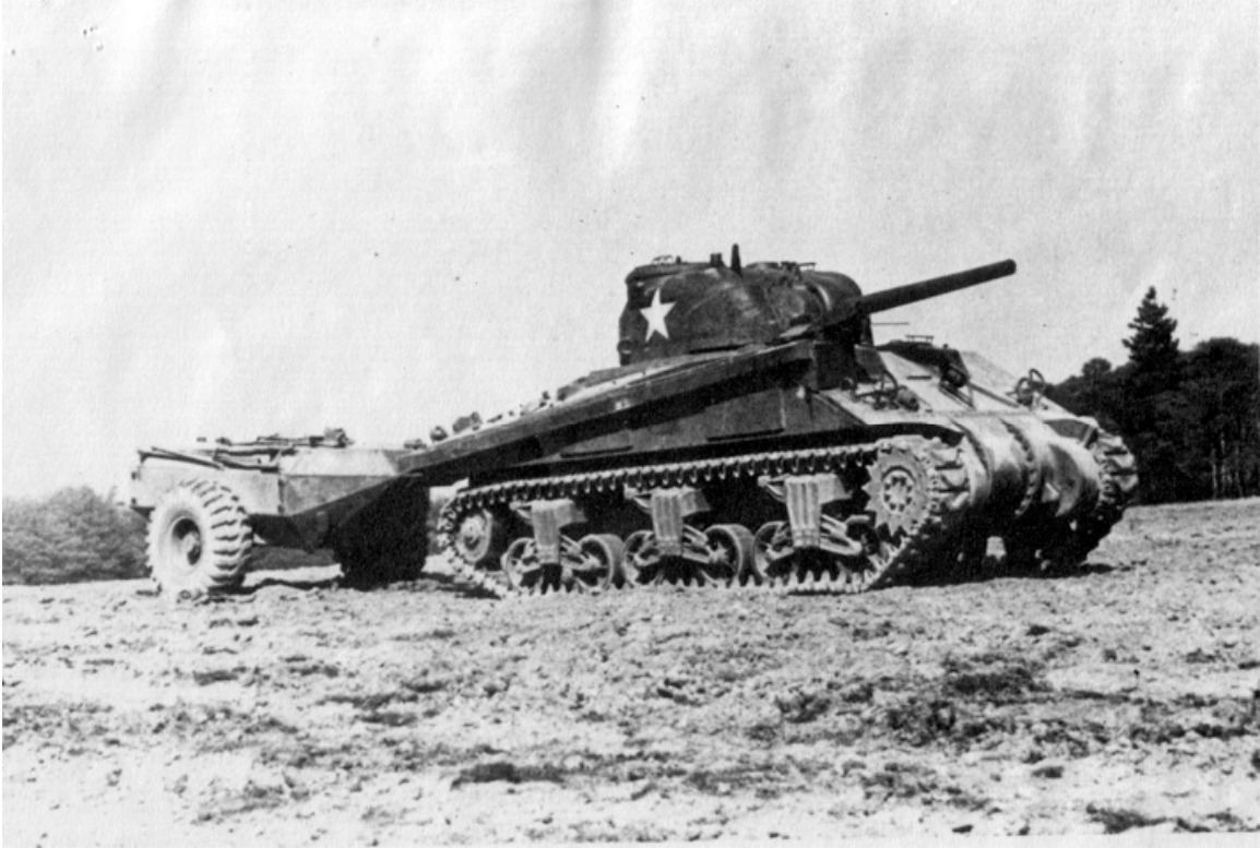
Army2: One of only four Sherman Crocodiles to enter American service. The nozzle is to the right of the bow gunner's hatch, and the trailer carries the fuel. (U.S. Army photo, records of the Armored Board)
