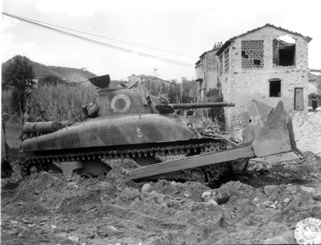
SC-194744: A 1st Armored Division tank dozer opens the way for a column in Italy in September 1944. (NARA, Signal Corps photo)
