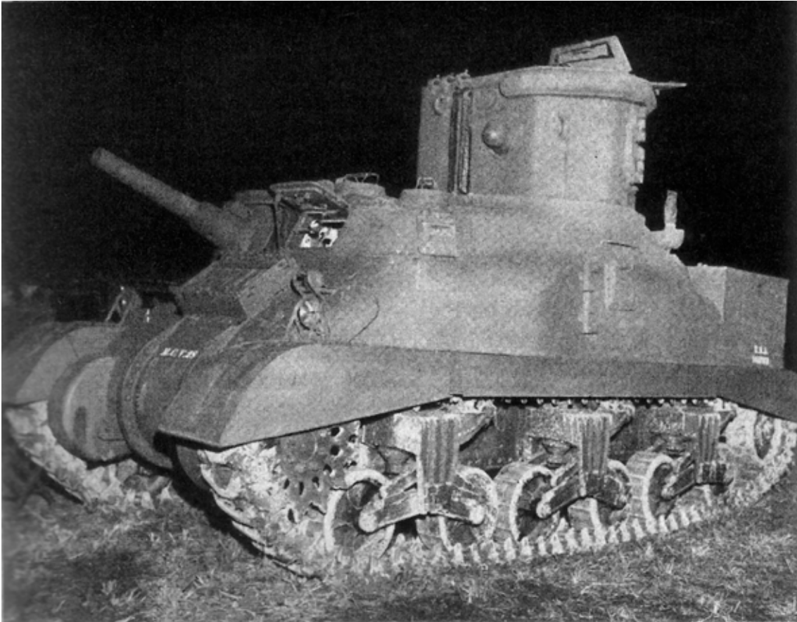
Army16: A 13 million-candlepower arc light projected through the vertical slit in the turret of the CDL tank. This U.S. Army CDL is based on an M3A1 medium tank. (U.S. Army photo)
