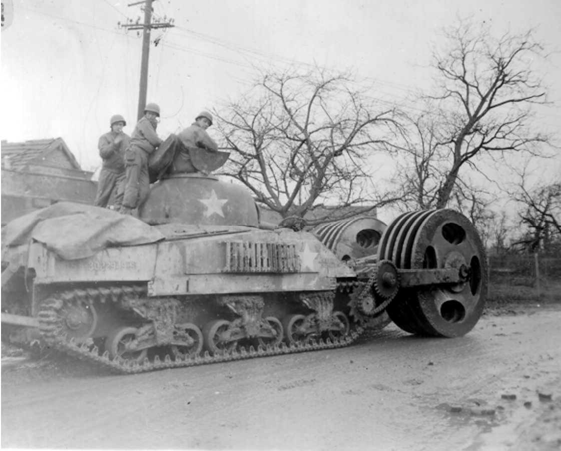
SC-242926: A 739th Tank Battalion (Mine Exploder) T1E3 "Aunt Jemima" (hint: stacked pancakes) clears a road near Beggendorf, Germany, in December 1944. (NARA, Signal Corps photo)
