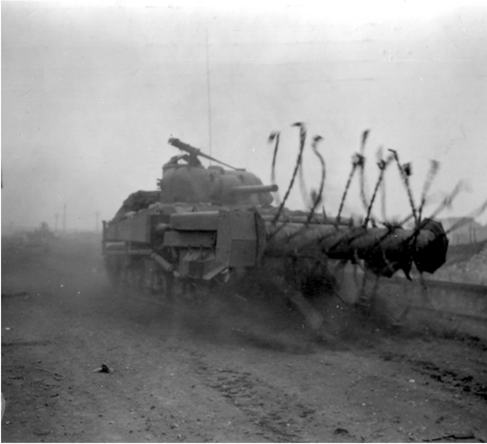
SC-195471: The Crab flail tank was the most important mine clearer in American service but was far from perfect. (NARA, Signal Corps photo)
