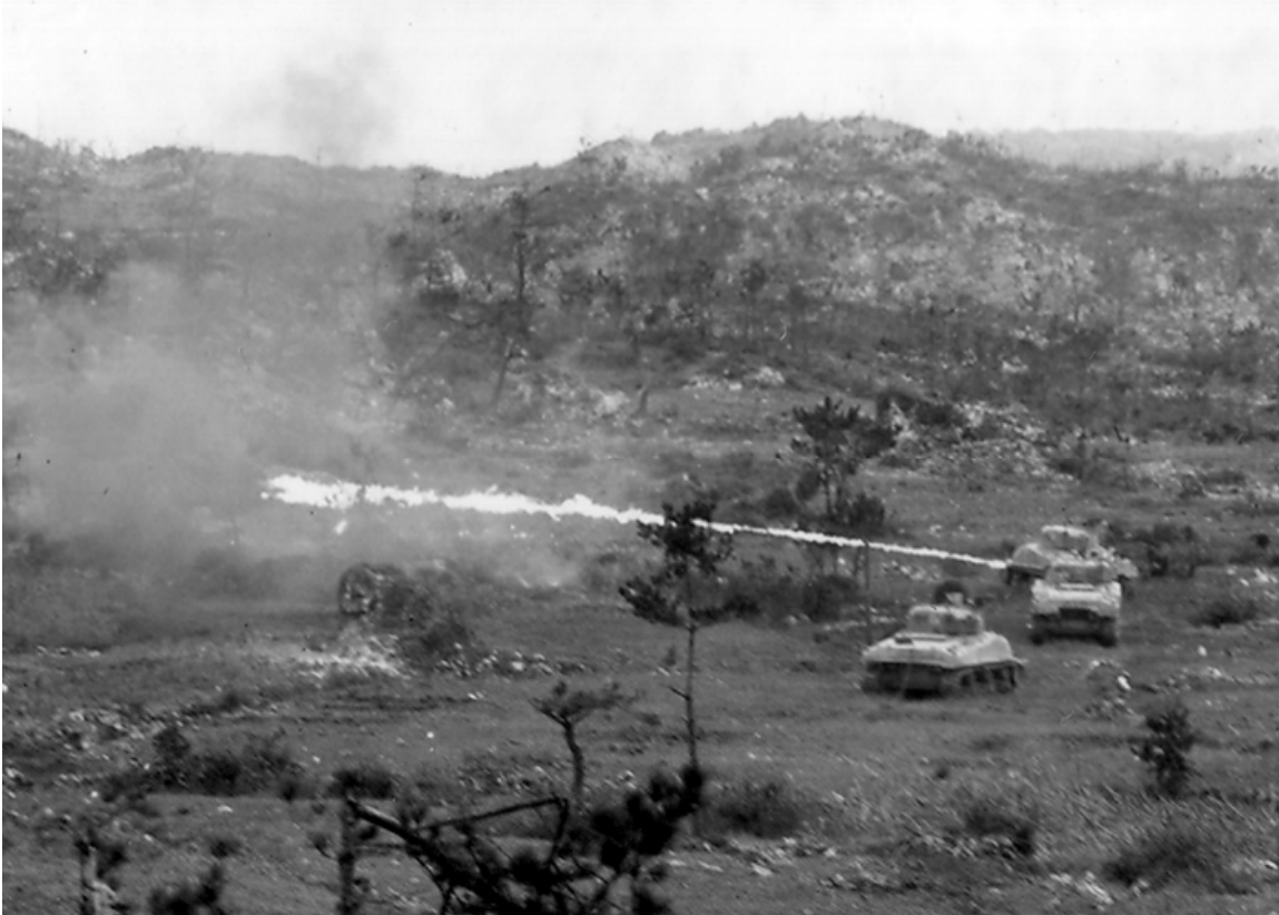
SC-209094: A Sherman with a bow-mounted flamethrower fires at a Japanese-occupied cave on Okinawa in June 1945. The relatively short range was not a problem in the Pacific because the Japanese lacked the bazooka-type weapons fielded by the Germans, which could kill a tank at about the same distance. (NARA, Signal Corps photo)
