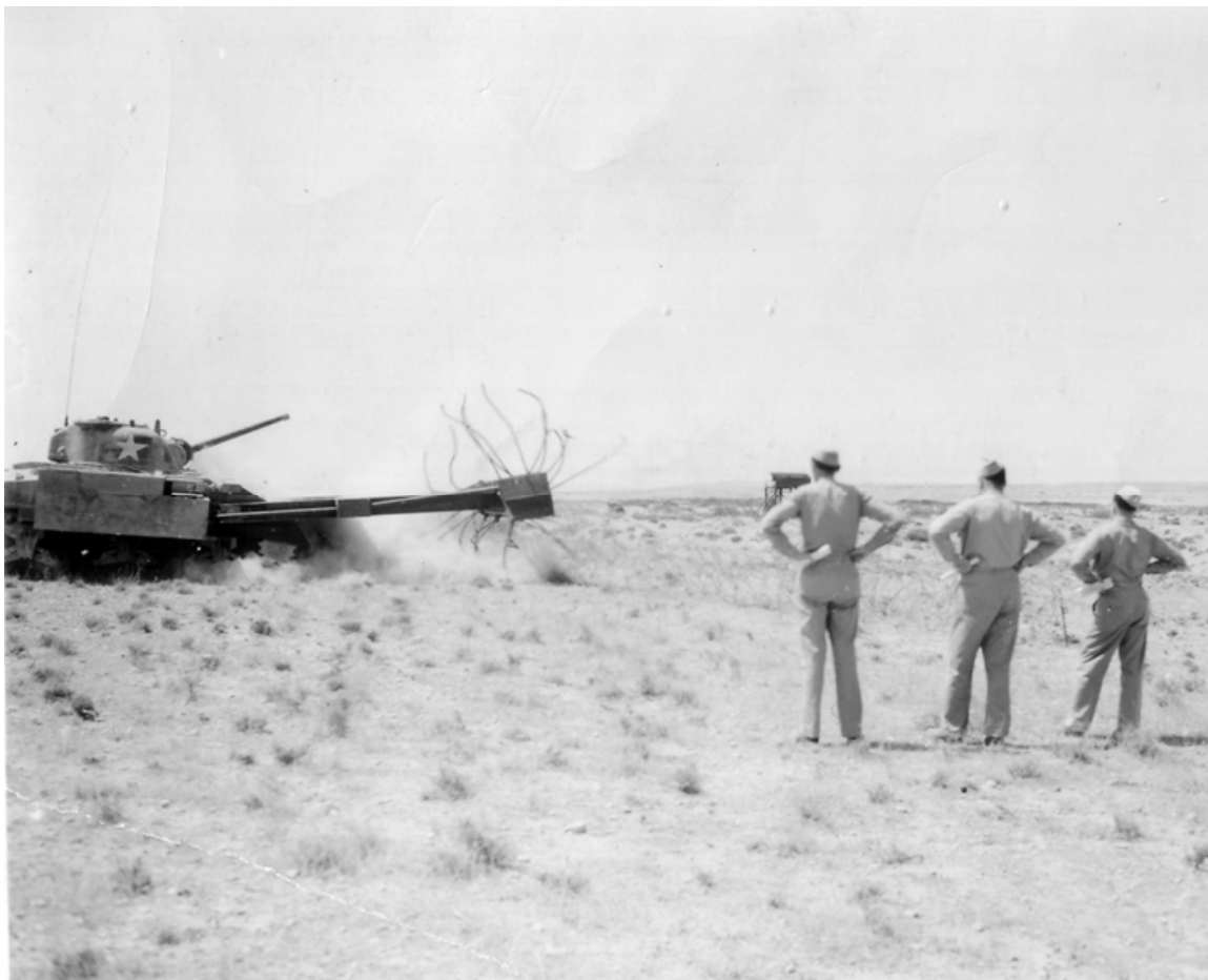
SC-190899: A Scorpion flail tank demonstration in North Africa in August 1943. Note the outboard engine on the right side. (NARA, Signal Corps photo)
