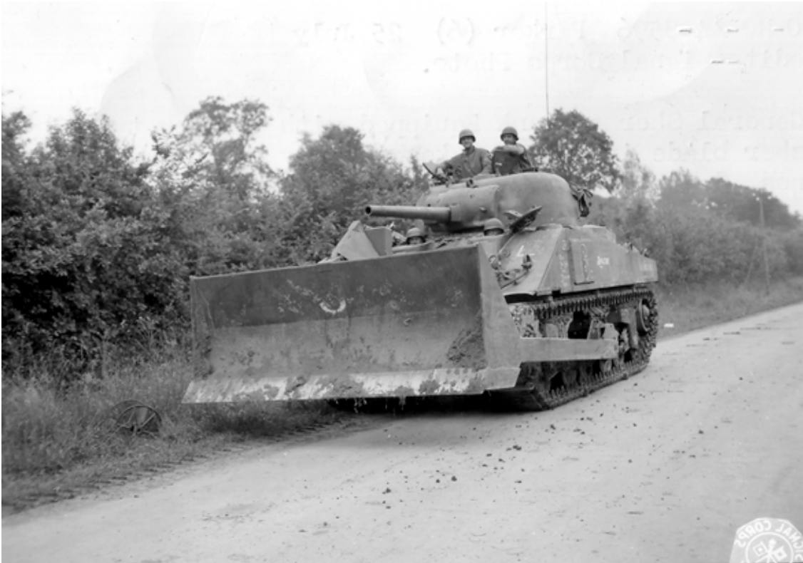
SC-191908-S: A Tank dozer in Normandy in July 1944. (NARA, Signal Corps photo)
