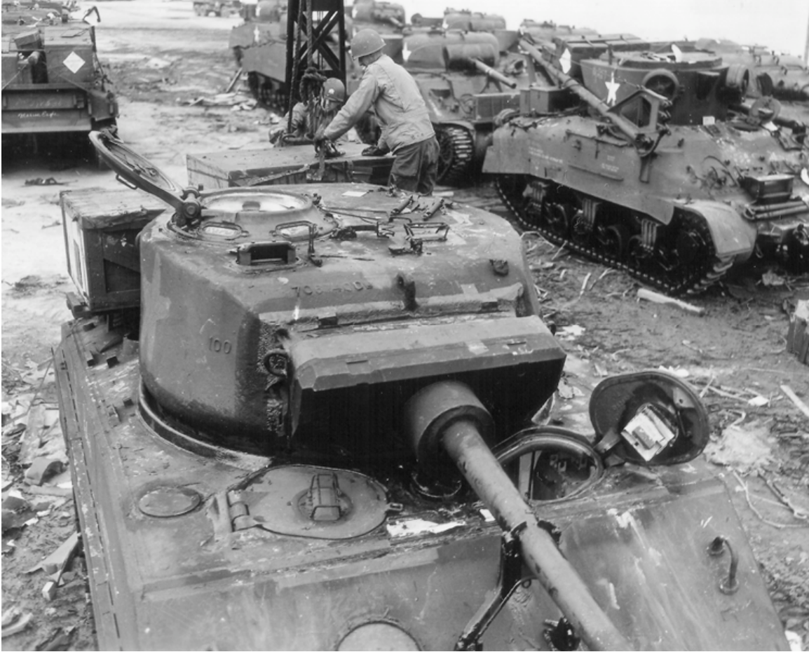
SC-196503: A newly arrived M4A3E2 Jumbo in November 1944 offers a good view of the commander's cupola also found on the 76mm M4 turret. The added loader's hatch is closed. Note the massively armored turret front, including the gun mantlet. The seam from the extra glacis armor is visible in front of the hull hatches. (NARA, Signal Corps photo)
