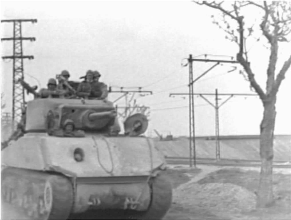
111-ADC-4025_3: Not satisfied with the Tiger-tank-thick glacis on the Jumbo, the 750th Tank Battalion poured a layer of concrete on top. (National Archives, Signal Corps film)
