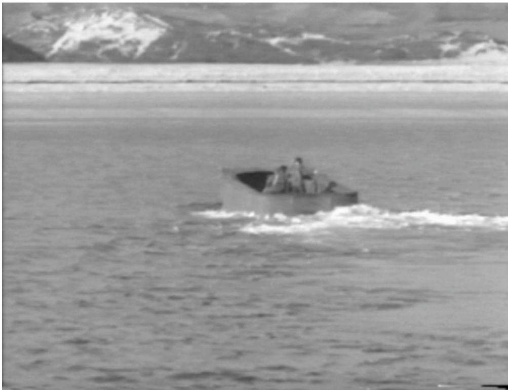
111-ADC-867_6: Under power, the screen provided no more than 3 feet of freeboard, which left the DD vulnerable to swamping by even modest waves. (NARA, Signal Corps film)
