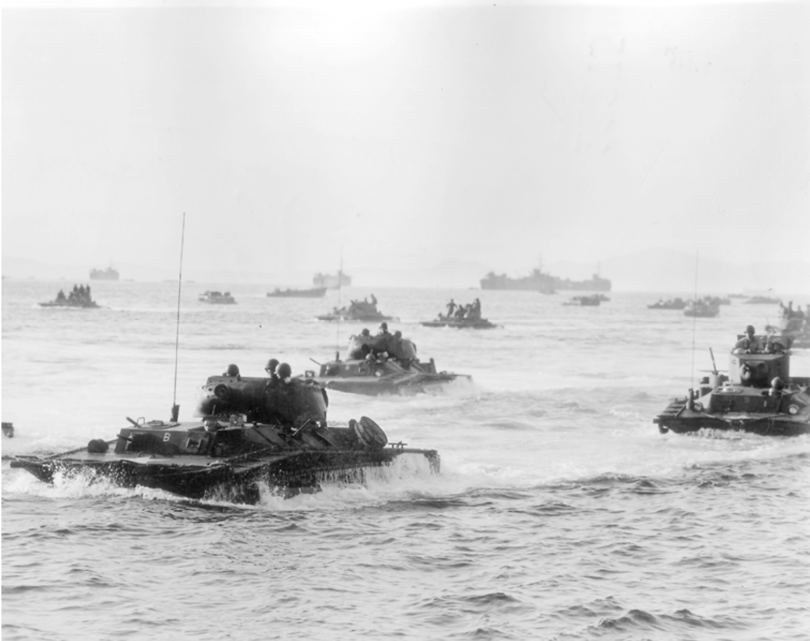
SC-206509: LVT(A)(4) (near left) and LVT(A)(1) (near right) amtanks, almost certainly from the 708th Amphibian Tank Battalion, head for the beach on Okinawa. Extra .30-caliber machine guns mounted at the side hatches of the LVT(A)(4)s are just visible. (NARA, Signal Corps photo)
