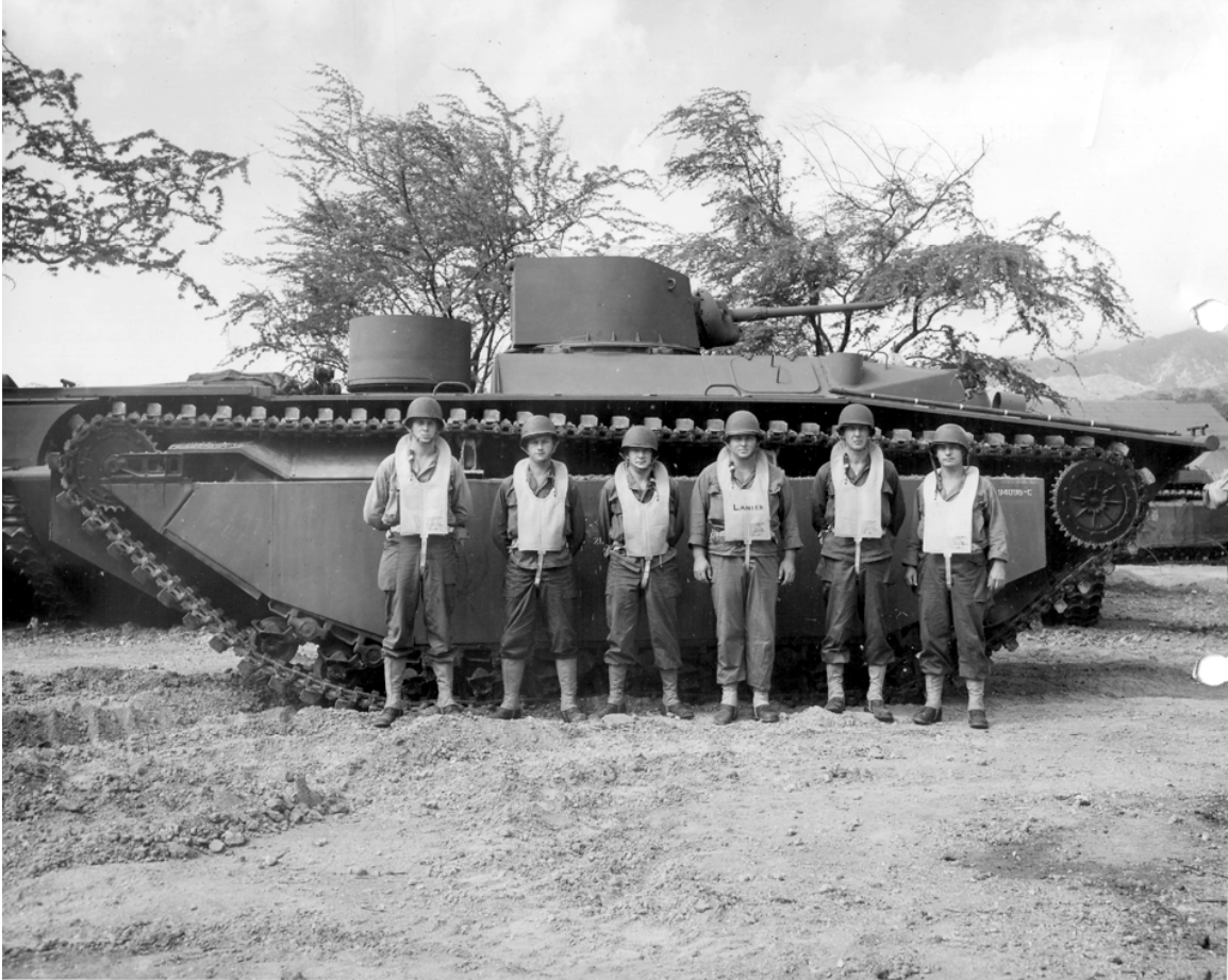
708th_2: An LVT(A)(1) amtank and crew. Note the M5 tank turret and, behind that, the right-side scarf mount (facing to rear) for a .30-caliber machine gun. (NARA, 708th Amphibian Tank Battalion records)
