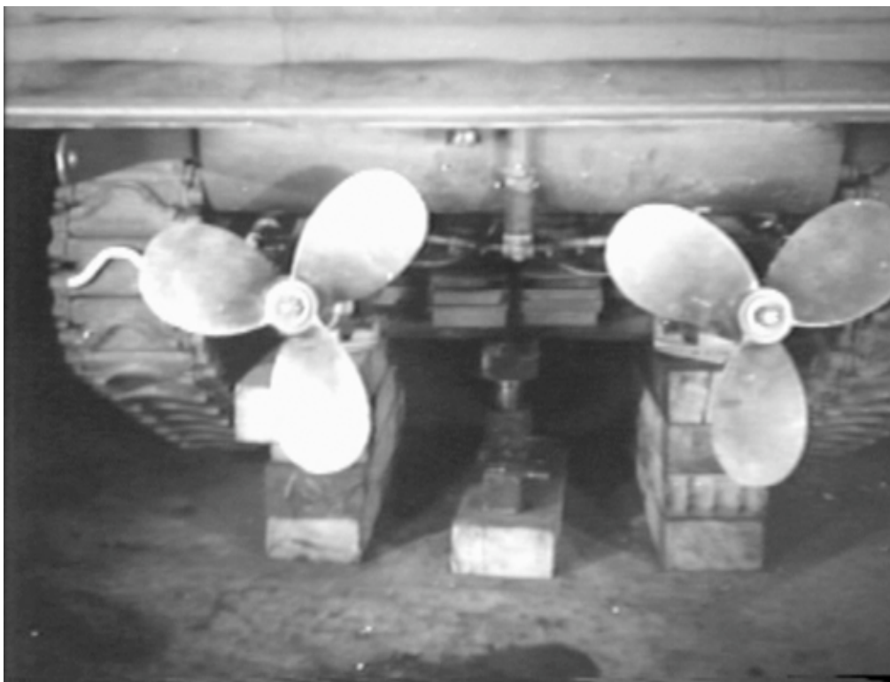
111-ADC-867_3: The propellers could be raised and lowered from inside the tank and pivoted from side to side to steer the vehicle. (NARA, Signal Corps film)
