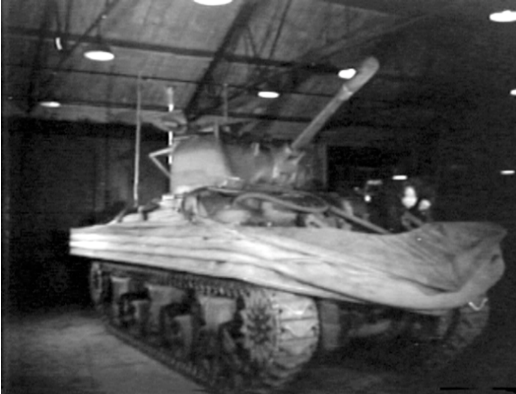
111-ADC-867_1: The DD Sherman with screens lowered. The hoses visible on the frontal armor supplied compressed air to inflatable tubes that raised the screen. One of the struts that locked the screen in place is visible in a folded position on the turret below the commander's hatch, and another is to the right of the bow gunner's position. (NARA, Signal Corps film)
