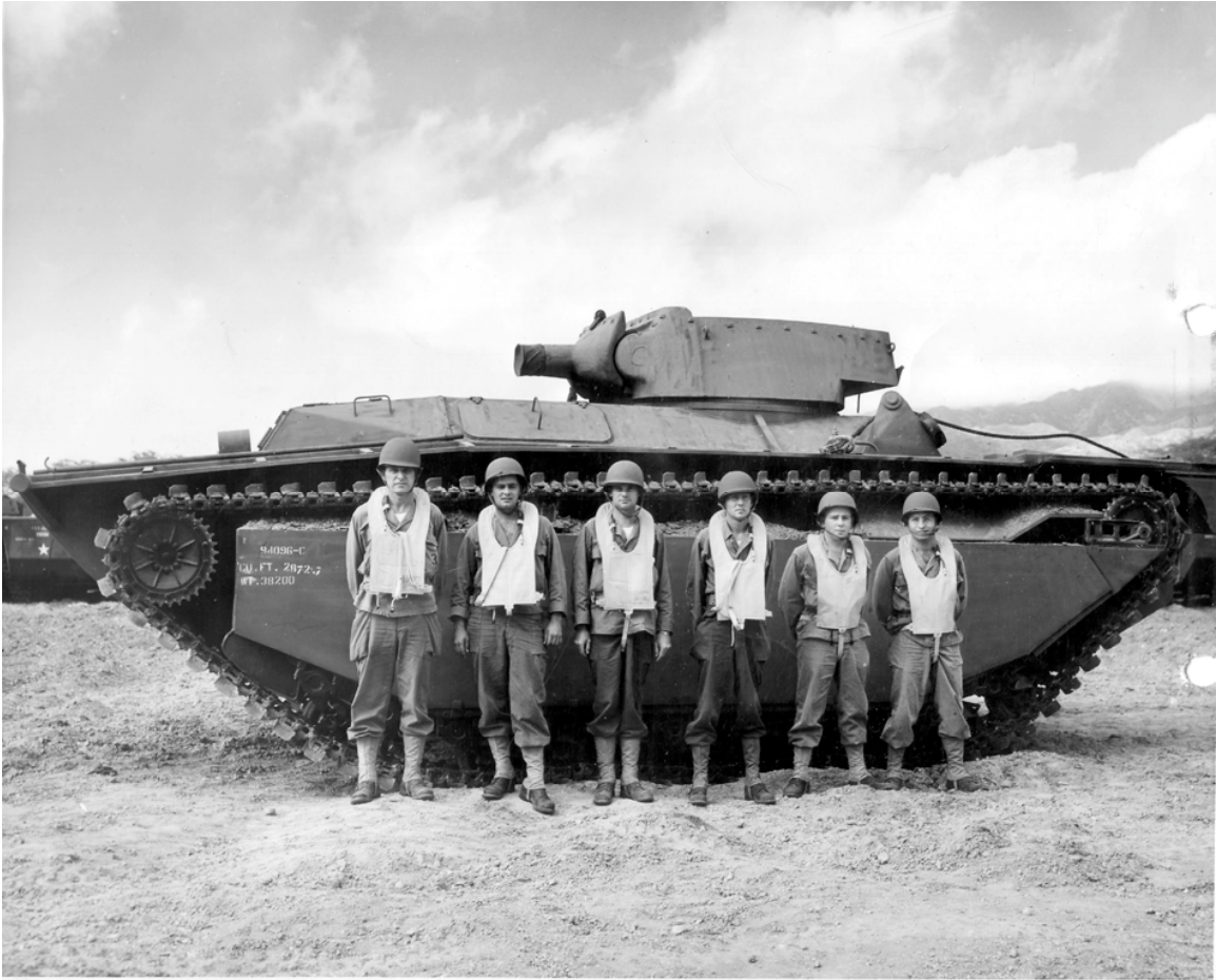
708th_1: An LVT(A)(4) and crew. This vehicle does not have the .50-caliber turret anti-aircraft machine gun mounted—the only weapon initially available for use against attacking infantry. (NARA, 708th Amphibian Tank Battalion records)
