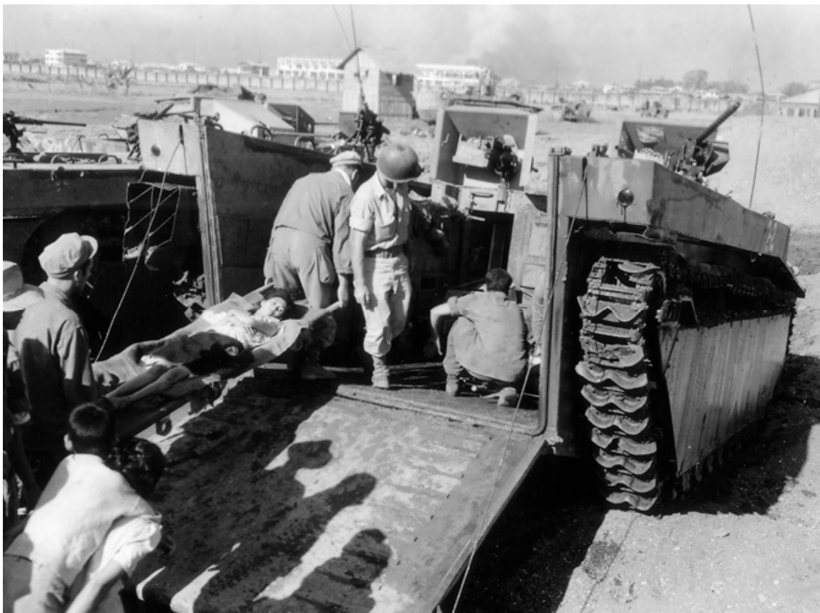
SC-202156: A view of the LVT(4)'s ramp, troop/cargo space, and machine gun positions. Note the scoops on the track blocks that enabled movement in water and the damage to the right track, possibly caused by hard surfaces on shore. (NARA, Signal Corps photo)
