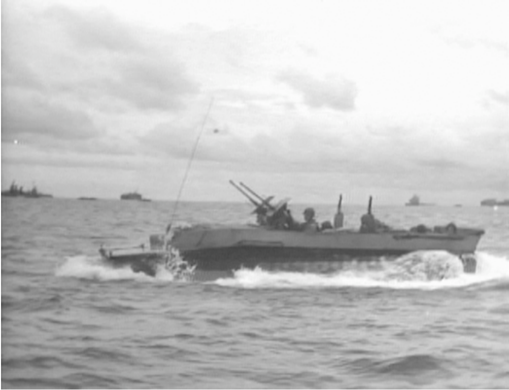
111-ADC-2460_1: An LVT(4) under way during the landings on Angaur in the Pelau Islands on 17 September 1944. The tracks provided the motive force in the water. (NARA, Signal Corps film)
