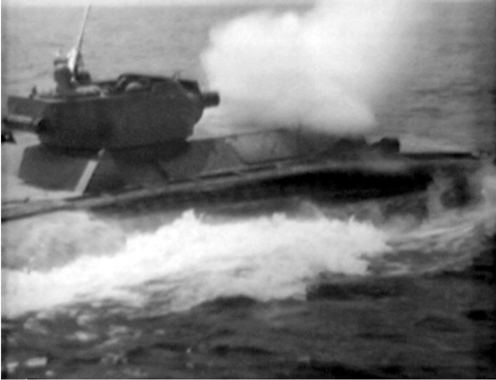
80-MN-4381_2: The LVT(A)(4) could lay down fairly accurate fire while afloat as long as the sea was relatively calm. This antank has the .50-caliber machine gun mounted. (NARA, Signal Corps film)
