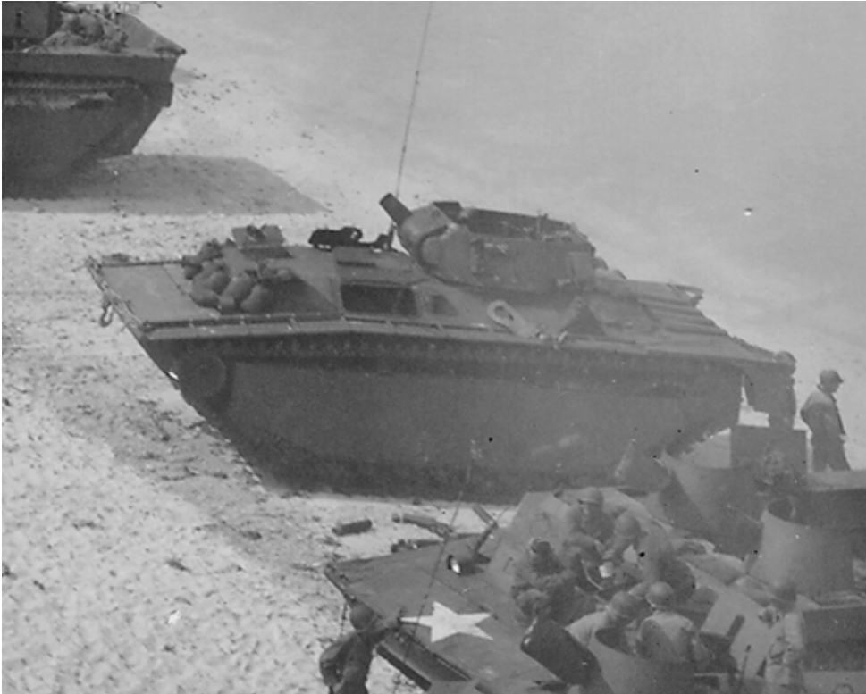
SC-205185: An LVT(A)(4) on Hokaji Shima, Ryukyu Islands, on 26 March 1945 reveals its open-topped turret, nearly identical to the one on the M8 assault gun. The amtank has a bow machine gun and sandbags for extra protection, and the main gun is elevated to fire indirectly. (NARA, Signal Corps photo)
