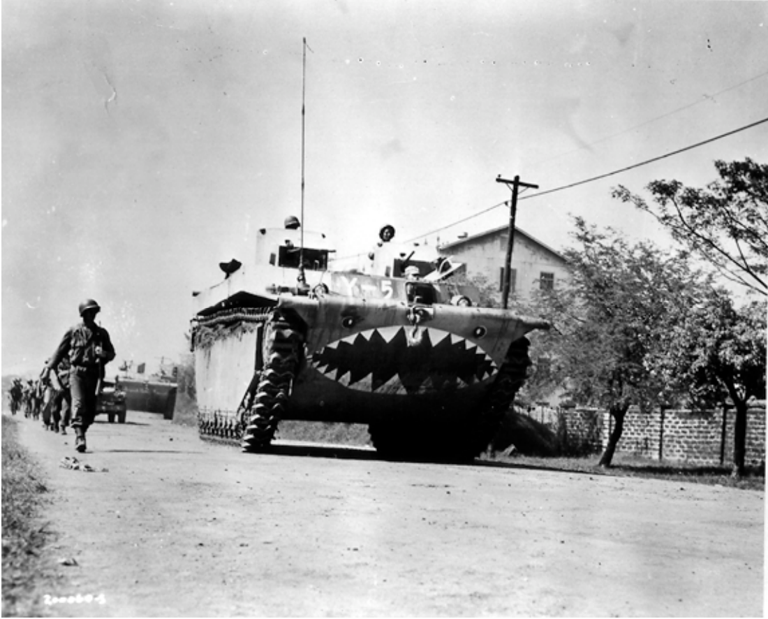
SC-200060-S: LVT(4)s approach Manila on 7 February 1945. Roads tended to damage the fragile tracks. (NARA, Signal Corps photo)
