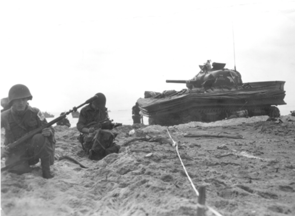
SC-246270: A DD Sherman of the 756th Tank Battalion crosses the landing beach during Operation Dragoon on 15 August 1944. The crew has already collapsed the skirt that converted the vehicle into an armored boat. (NARA, Signal Corps photo)
