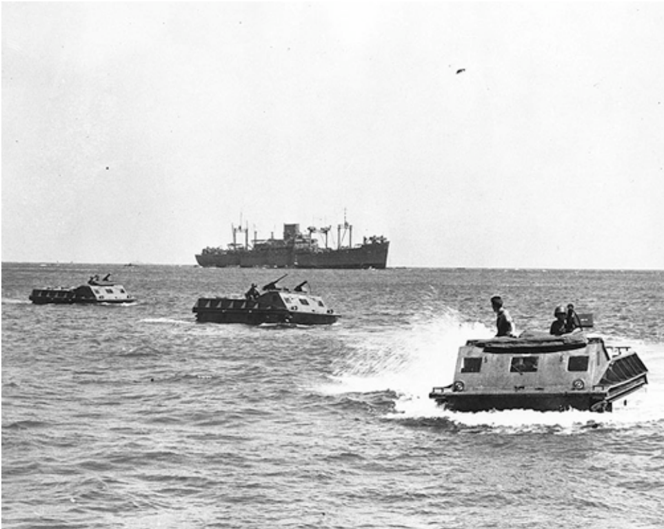
NH97749: LVT(1)s, these belonging to the Marine Corps, head for the beach at Guadalcanal in August 1942. The amtracs only carried cargo during this, their first appearance. (U.S. Navy photo)
