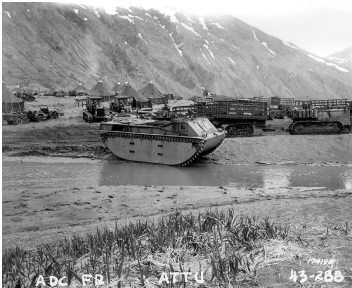
SC-174198: The LVT(1) Alligator did not serve in battle with the Army, but even official sources sometimes referred to later models by that name. The side pontoons on the LVT(1) were taller and covered more of the suspension system than on models used by Army battalions. (NARA, Signal Corps photo)
