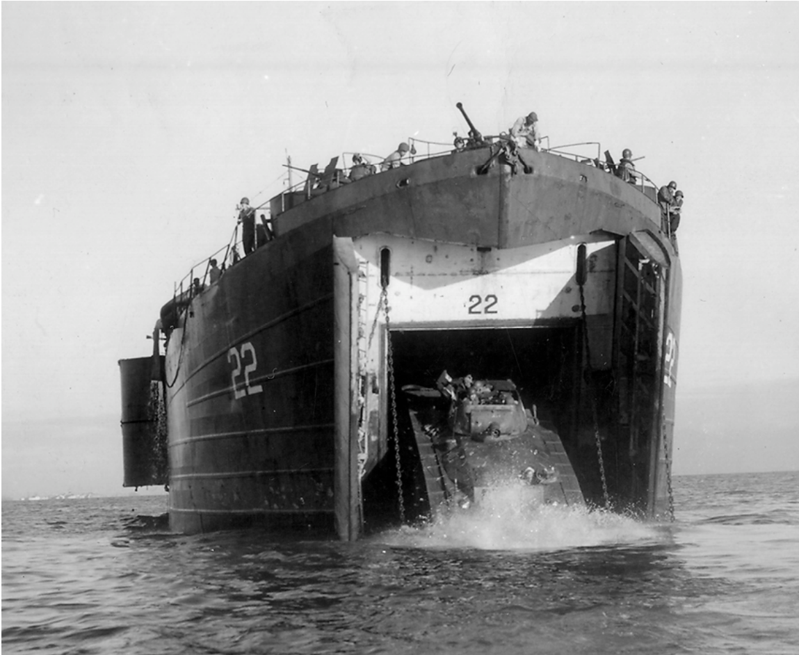
SC-200500-S: An LVT(A)(4) exits an LST in deep water to join the rest of the first wave off Luzon on 9 January 1945. (NARA, Signal Corps photo)
