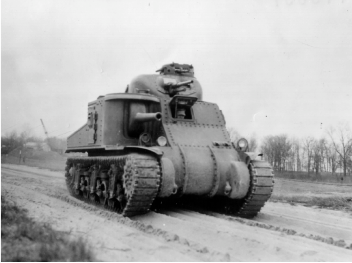
SC-118857: One of the first M3 medium tanks undergoes testing at Aberdeen Proving Ground in April 1941. Note the holes for fixed machine guns beside the left headlamp, the short-barreled 75mm Gun M2 without gyrostabilizer, and the absence of stowage bins on the back deck that were added to later vehicles. (NARA, Signal Corps photo)
