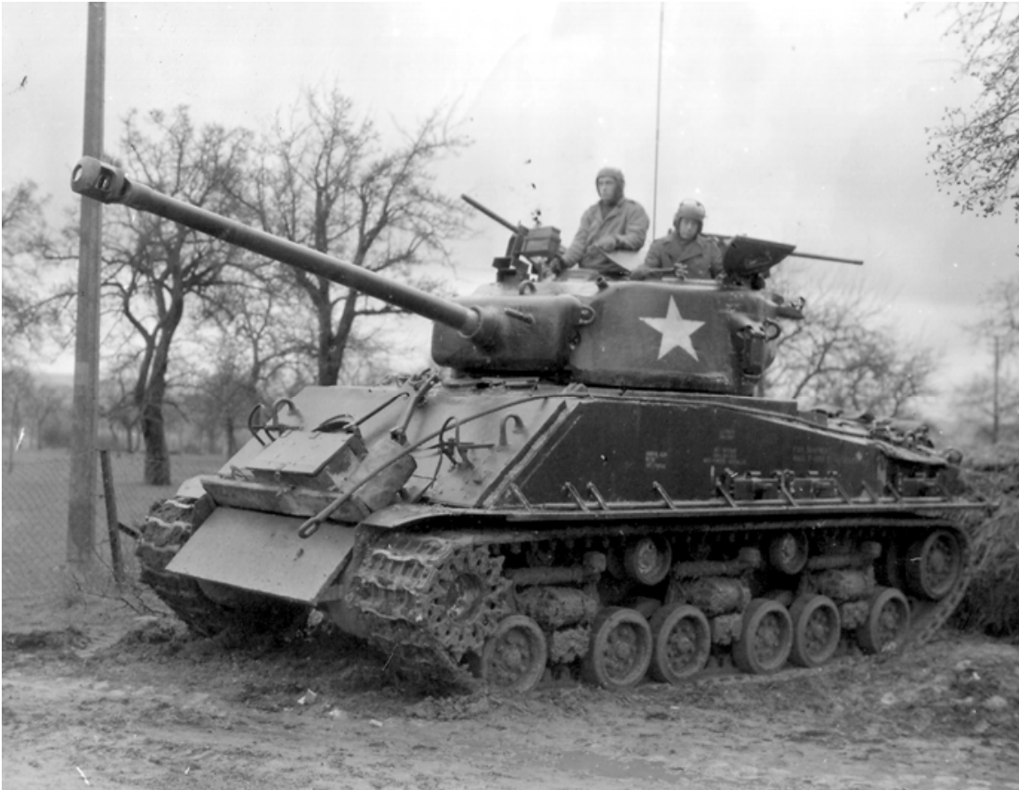
SC-203698: An M4A3E8 with a 1-inch add-on armor plate welded to the glacis. The loader's position is fitted out with an old-style commanders ring hatch. (NARA, Signal Corps photo)
