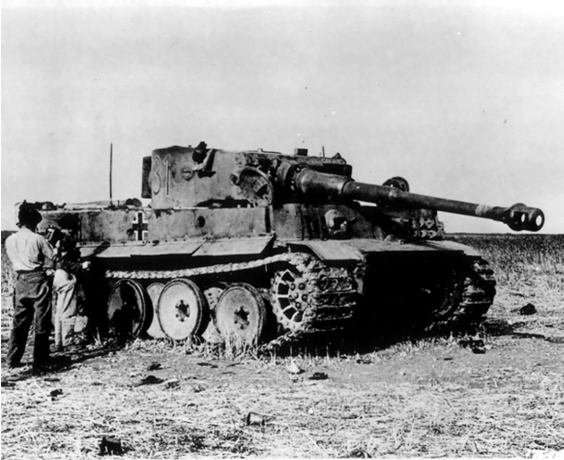
SC-175484: A Mark VI knocked out by a British Sherman in Tunisia in April 1943. An M4 gunner usually had to catch a Tiger with a shot from the flank, as in the case, or the rear in order to score a kill. (NARA, Signal Corps photo)
