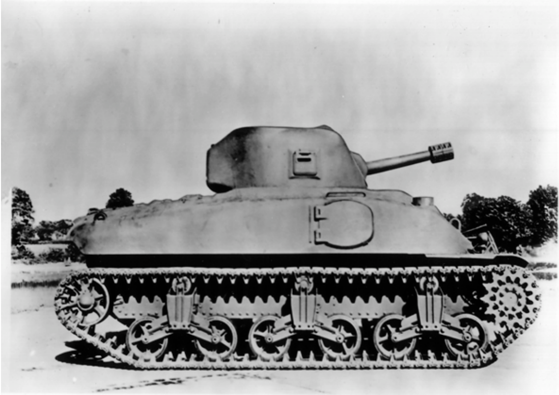
SC-130896: The T6 medium tank pilot was completed in September 1941, nine months after the first M3 Lee. (NARA, Signal Corps photo)
