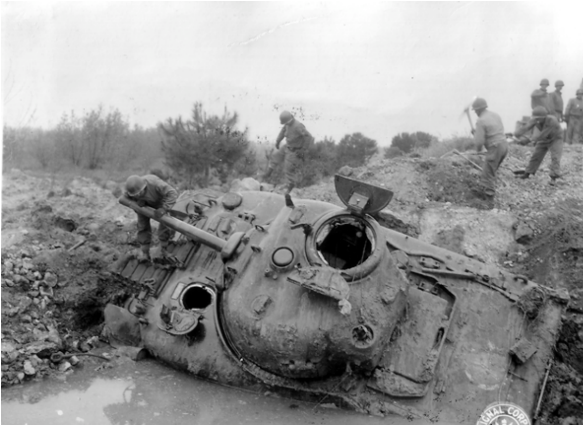
SC-189595: An unfortunate incident involving a bomb crater near Littoria, Italy, provides a top view of an M4A1. All three members of the turret crew had to make it out of the single hatch in case the tank caught fire. Periscopes are visible in the driver's and commander's hatches. (NARA, Signal Corps photo)
