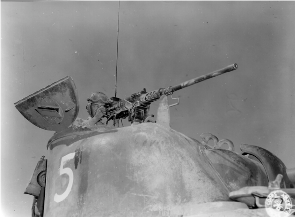
SC-239946: Firing the .50-caliber machine gun mounted beside the commander's hatch on an early model M4. This photo offers a clear view of the blade-style sighting vane the commander could use to roughly aim the main gun at a target. (NARA, Signal Corps photo)
