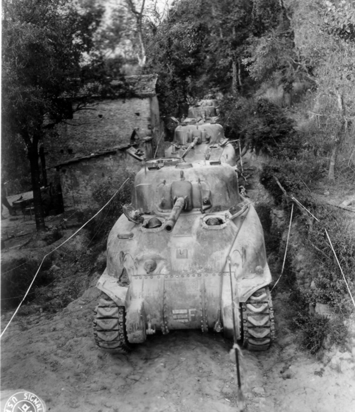
SC-190188: M4A1s from the 760th Tank Battalion near Turo, Italy, on 12 May 1944. The original hatches for the driver and bow gunner were an extremely tight fit. The lead tank has appliqué armor over the gunner's position. (NARA, Signal Corps photo)
