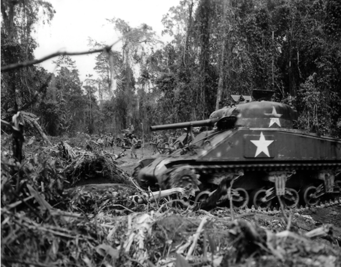
SC-188332: An M4 with the 56-degree glacis operates with the Americal Division on Bougainville in February 1944. This tank has appliqué armor in front of the hull hatches and over the sponson ammo racks (one on the left side and two on the right). It also has extra armor around the lower part of the turret, a modification common in the Pacific and possibly inspired by the Japanese practice of throwing explosive charges onto the deck. (NARA, Signal Corps photo)
