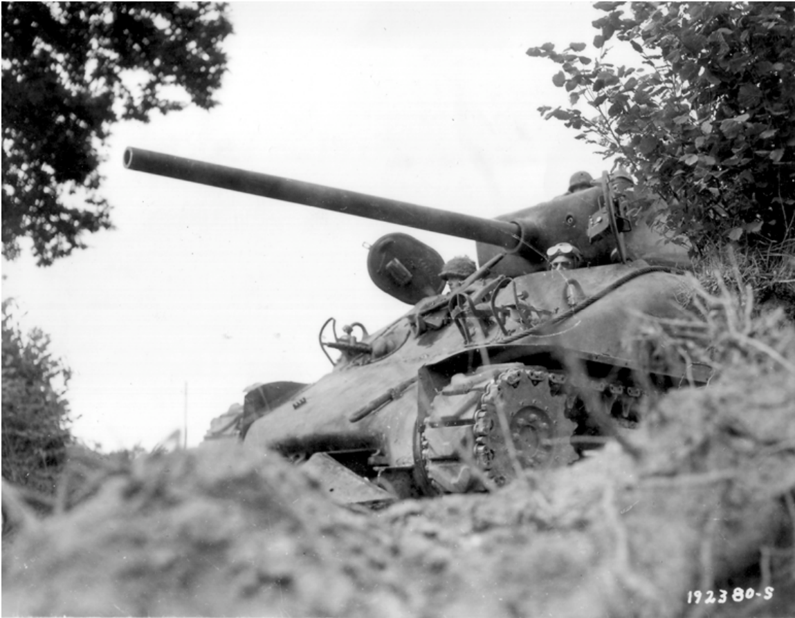
SC-192380: One of the first M4A1s (76mm) to see action in Normandy in August 1944. This one belongs to the 33d Armored Regiment, 3d Armored Division. The Signal Corps caption claims the new gun was known as the "hole puncher." (NARA, Signal Corps photo)
