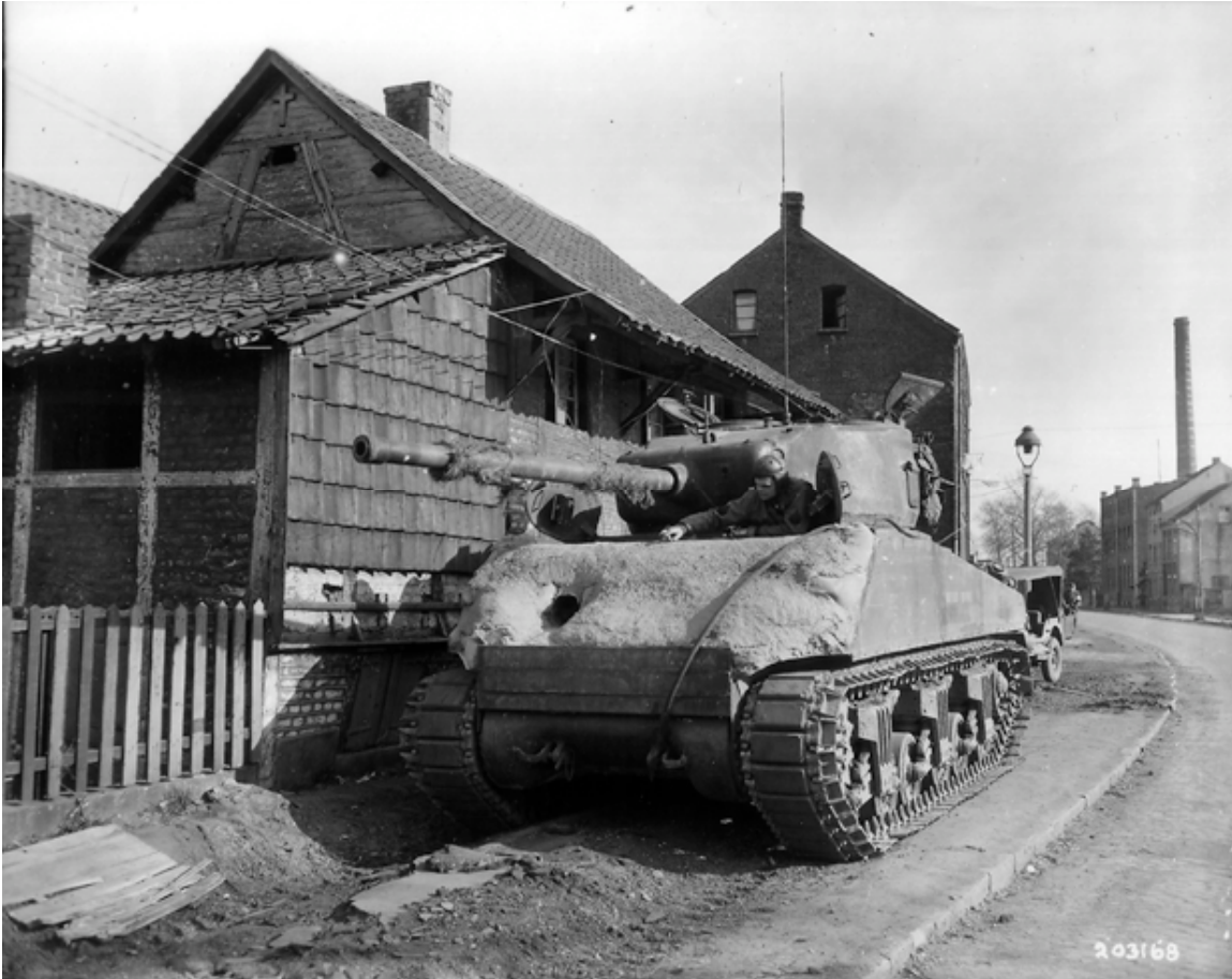
SC-203168: A 2d Armored Division M4A3 (76mm) displays another field expedient armor: a layer of concrete poured on the glacis. Experiments conducted by the 709th Tank Battalion in February 1945 indicated that poured concrete did not stop bazookas from penetrating the armor plate, but that it did reduce the splash of molten steel inside the tank caused by the warhead to "negligible" proportions. (NARA, Signal Corps photo)
