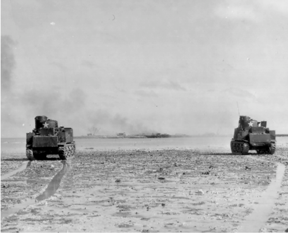
SC-183581: M3 tanks shell the Japanese at King's Wharf, Makin Atoll, on 21 November 1943. These Lees belong to Company A, 193d Tank Battalion. The lower elements of the wading stacks are still mounted. (NARA, Signal Corps photo)
