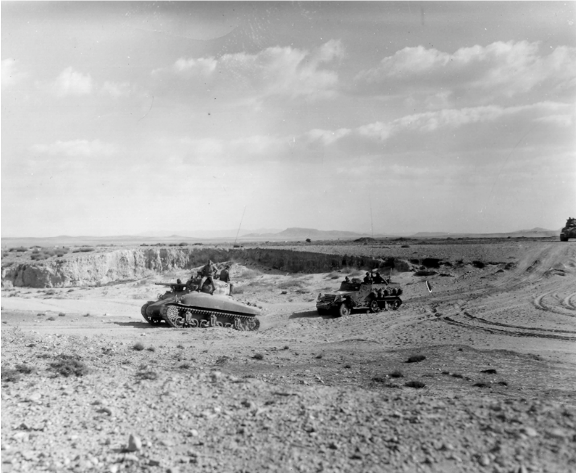
SC-170176: This almost certainly is part of Lt. Col. Louis Hightower's 2d Battalion retreating toward Sbeitla on 14 February 1943. An M4A1, recognizable by its smoothly curving cast hull, pulls a halftrack across a dry riverbed near Sidi bou Zid. (NARA, Signal Corps photo)
