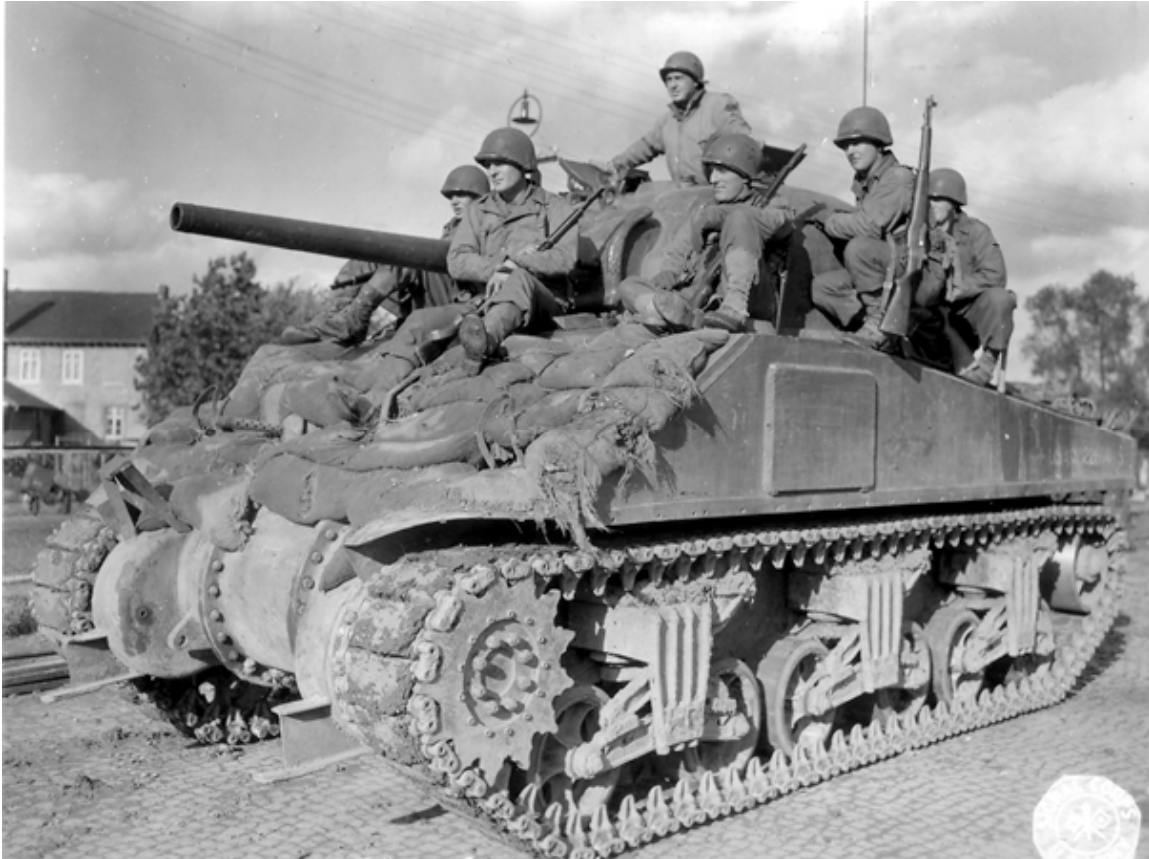
SC-195693: Tankers resorted to field expedients to reduce the likelihood of a penetration, at least by the ubiquitous German bazooka-style weapons. They first turned to sandbags during the fighting in Normandy; tests offered mixed results as to whether the bags worked, but they made tankers feel safer. Here, a 3d Armored Division Sherman displays a typical sandbagging job near Stolberg, Germany, on 14 October 1944. (NARA, Signal Corps photo)
