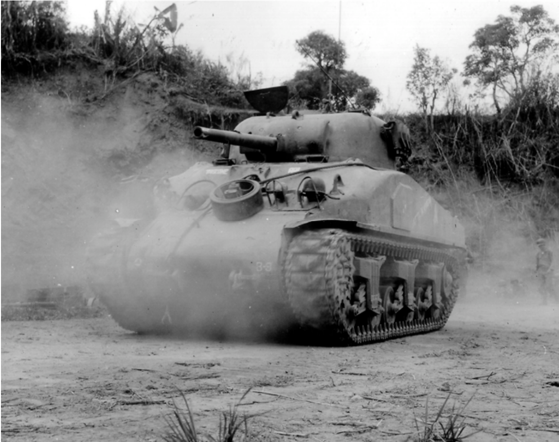
SC-208550: The composite hull, which mated a cast glacis with a welded main hull, was produced in limited numbers. (NARA, Signal Corps photo)
