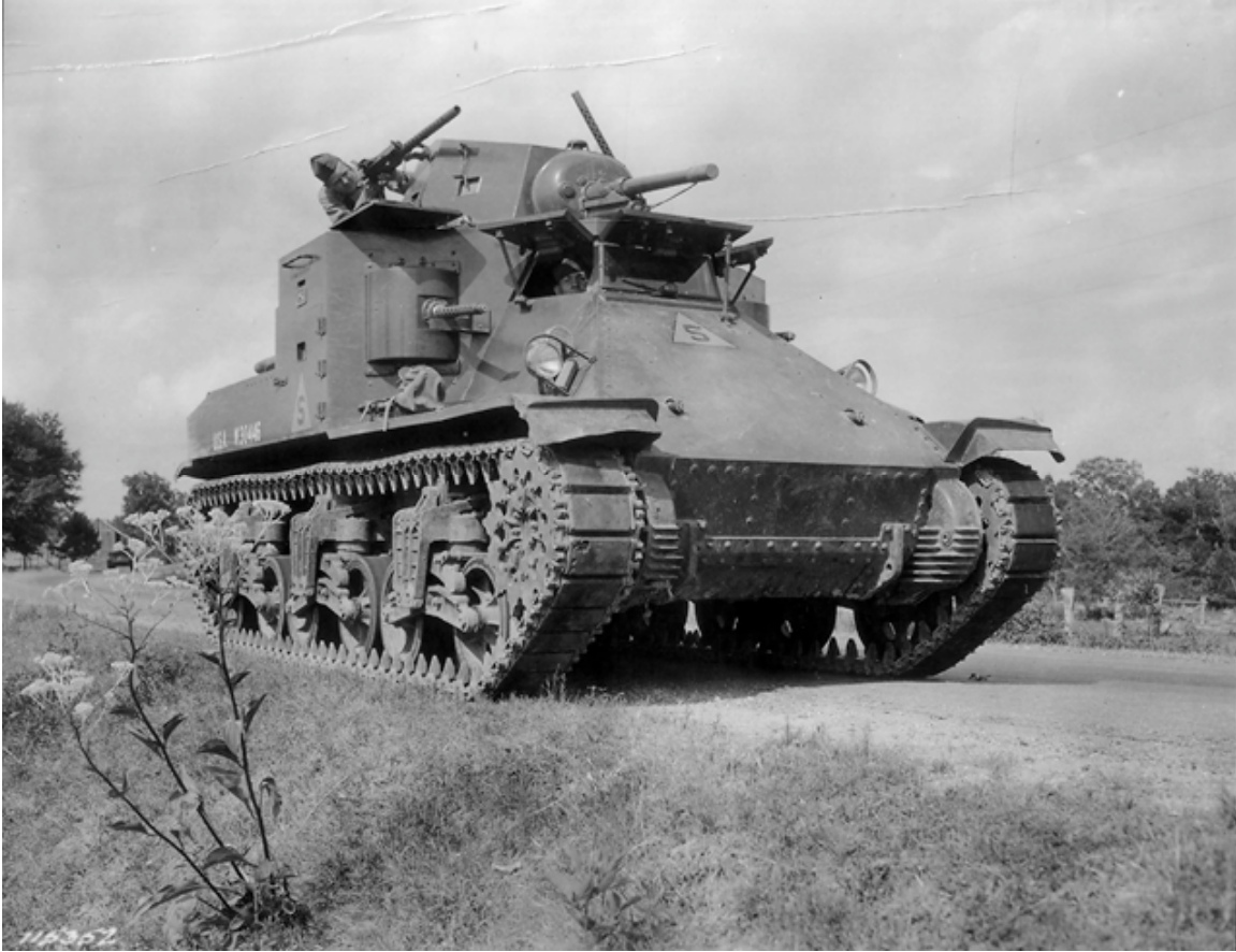
SC-115352: An M2A1 medium tank belonging to the 67th Infantry Regiment (Tanks) in 1940. The M2A1 had slightly thicker armor than the M2 and a supercharger on the engine to boost horsepower. Note the two fixed machine guns in the lower glacis armor. The vehicle passed on its chassis, the suspension arrangement, the power train, and much of its superstructure design to the M3. (NARA, Signal Corps photo)
