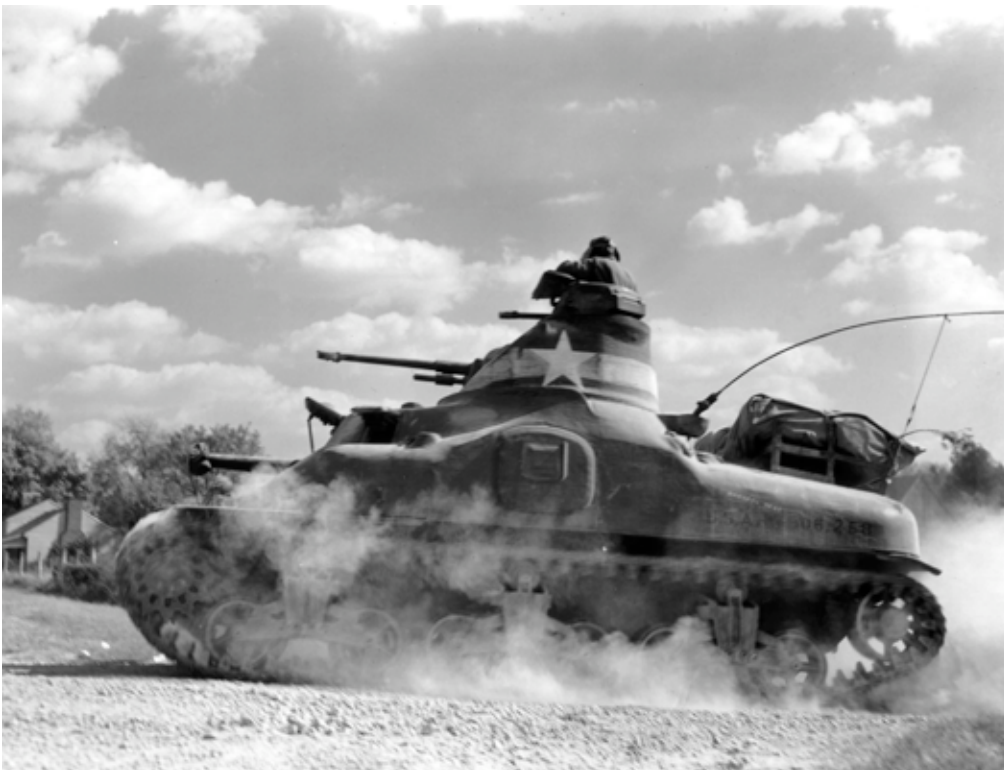
SC-169063: The rounded contours of the M3A1 with cast hull. (NARA, Signal Corps photo)
