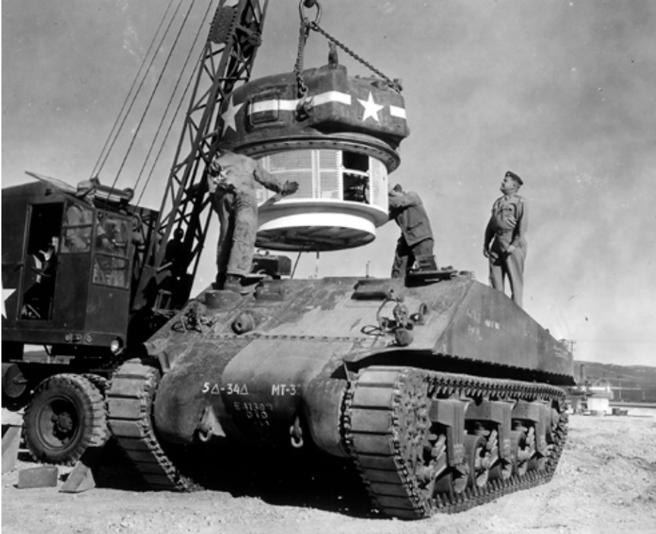
SC-186633: The turret basket of an M4 tank from the 34th Armored Regiment, 5th Armored Division. This tank has early vision blocks but a cast final drive housing. (NARA, Signal Corps photo)
