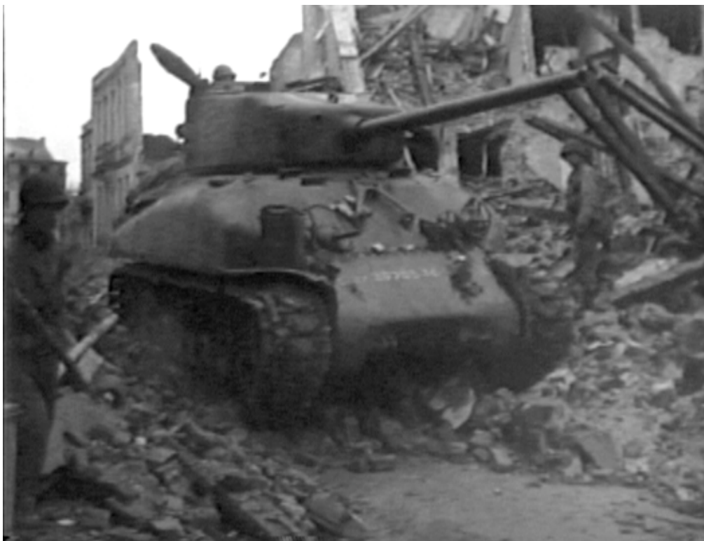
111-ADC-9704_2: A better view of the M4A1 (76mm), again belonging to the 3d Armored Division; this tank is part of the force that captured Cologne in March 1945. (NARA, Signal Corps film)
