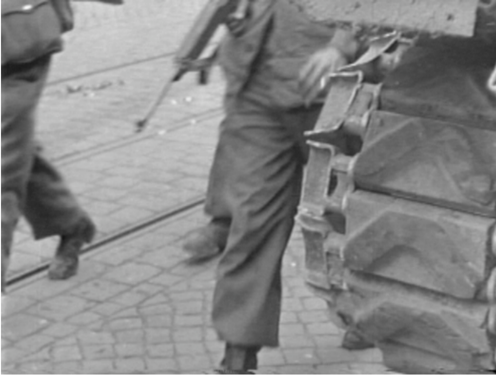
111-ADC-4025_1: A close-up view of track grousers, with their curved-edge construction that inspired the nickname "duckbills". (NARA, Signal Corps film)
