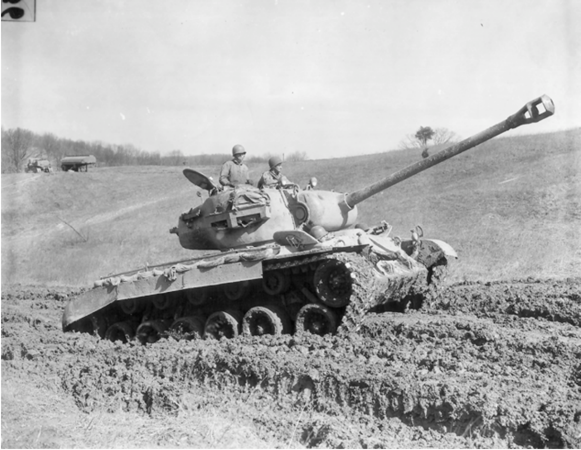
SC-204486: The new M26 heavy tank at Aberdeen Proving Grounds. The torsion-bar suspension system became standard on American tanks for decades to come. (NARA, Signal Corps photo)
