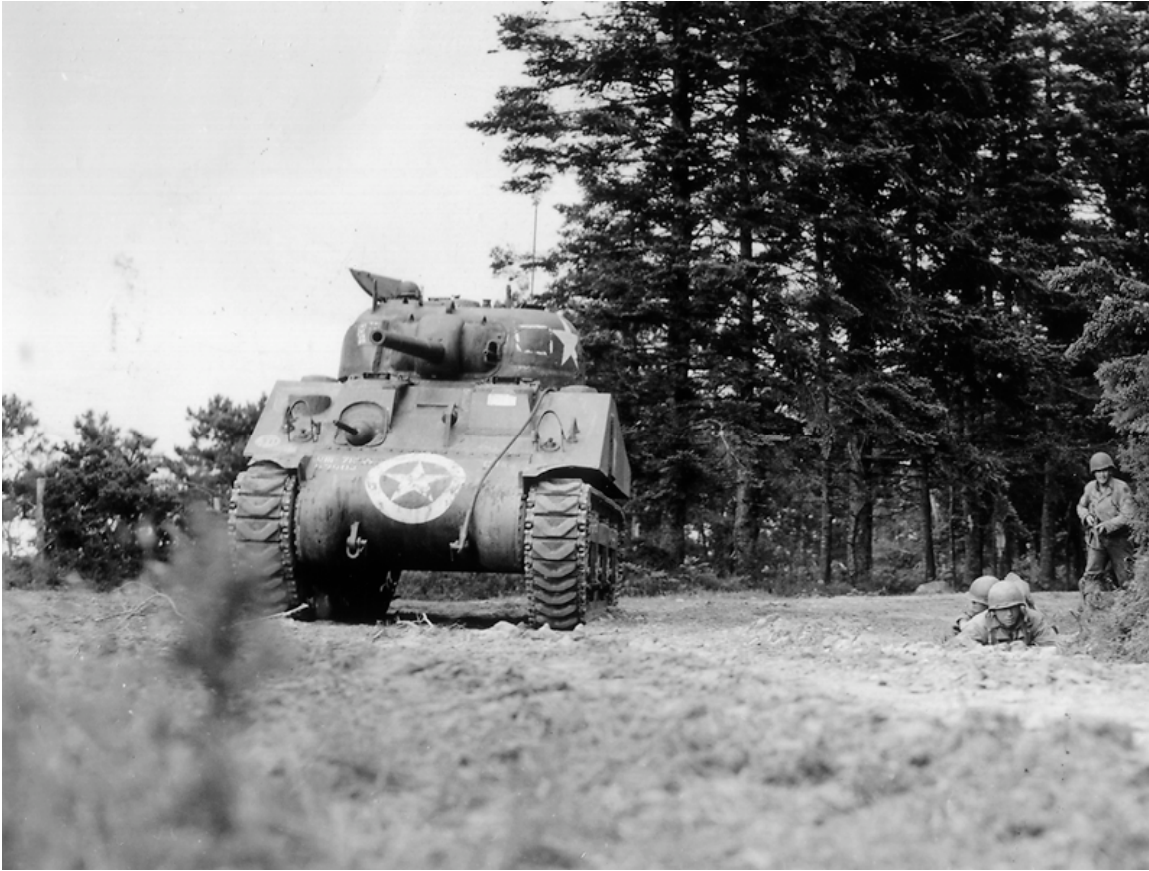
SC-191353: A venerable 712th Tank Battalion M4 advances with riflemen near St. Jores, France, on 7 July 1944. The tank displays the elimination of the hatch shot traps accomplished by welding angled iron plates in front of them. It also has appliqué armor on the right turret side over the gunner's position. (NARA, Signal Corps photo)
