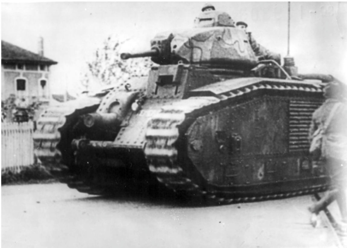
SC-119303: The French Char B1 bis heavy tank carried its 75mm gun in the hull. The upper turret sported a 47mm gun and coaxial machine gun. (NARA, Signal Corps photo)
