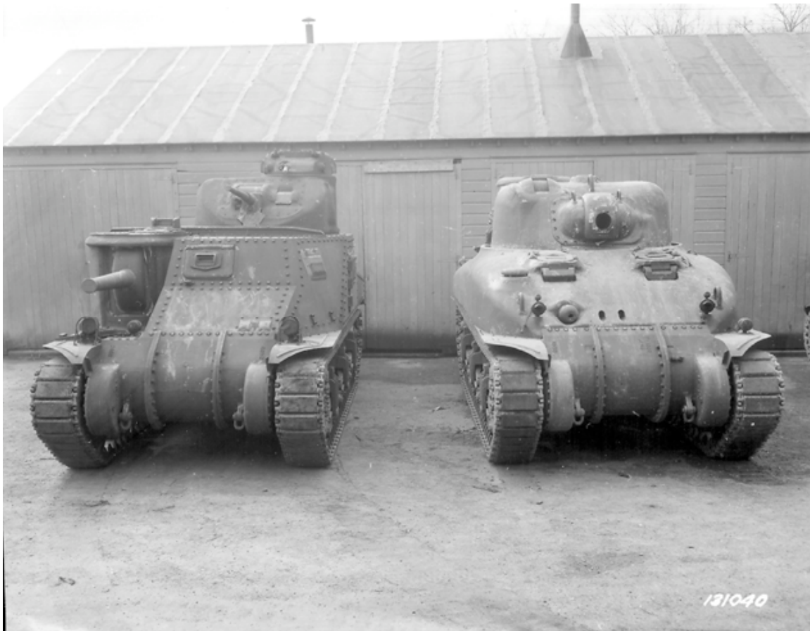
SC-131040-R: The M3 and new M4A1 medium tanks in spring 1942. The early M4A1 had solid vision blocks for the driver and bow gunner instead of periscopes. The bulge atop the M4A1 turret is an early version of the main gun sight; the gun itself is missing. (NARA, Signal Corps photo)
