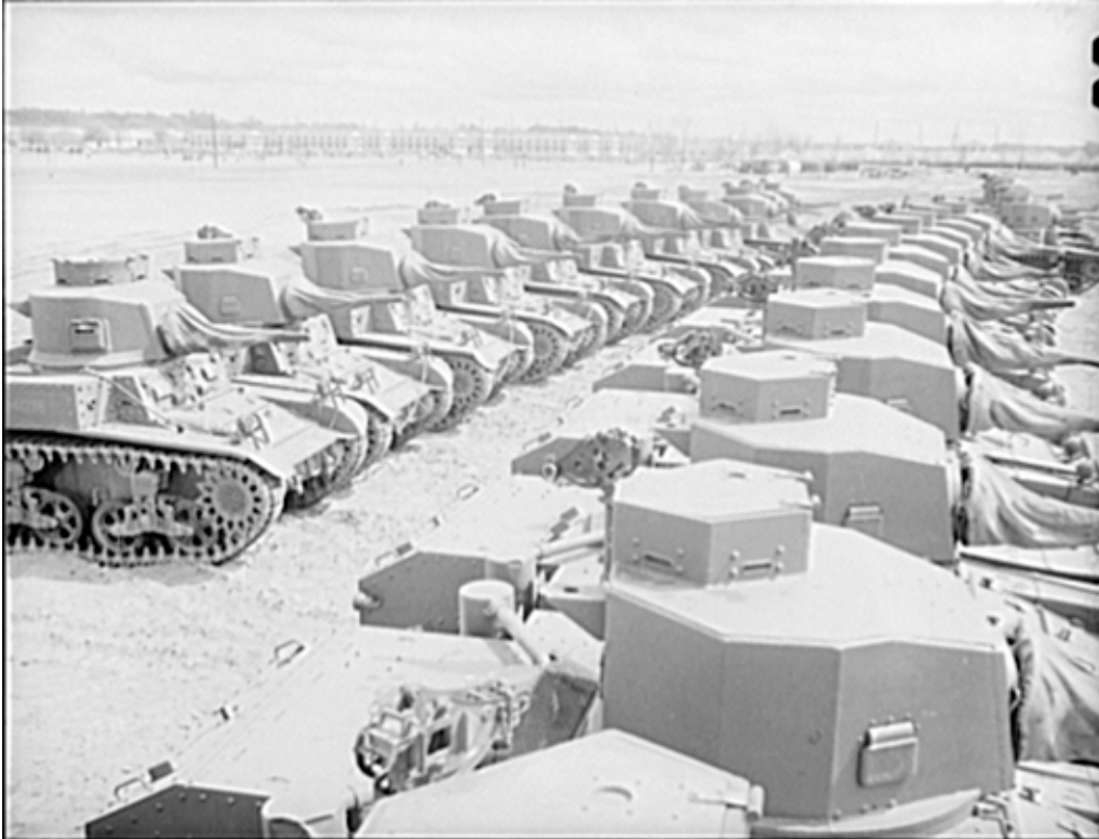
8b02792u: Evolution of the early M3 turret: Near right is the seven-sided welded turret that almost immediately replaced a similar riveted model. Near left is the successor welded homogeneous steel turret. This picture also offers a view of the M3's armored back deck, which was 3/8-inch thick. (Library of Congress, Prints & Photographs Division, FSA-OWI Collection)
