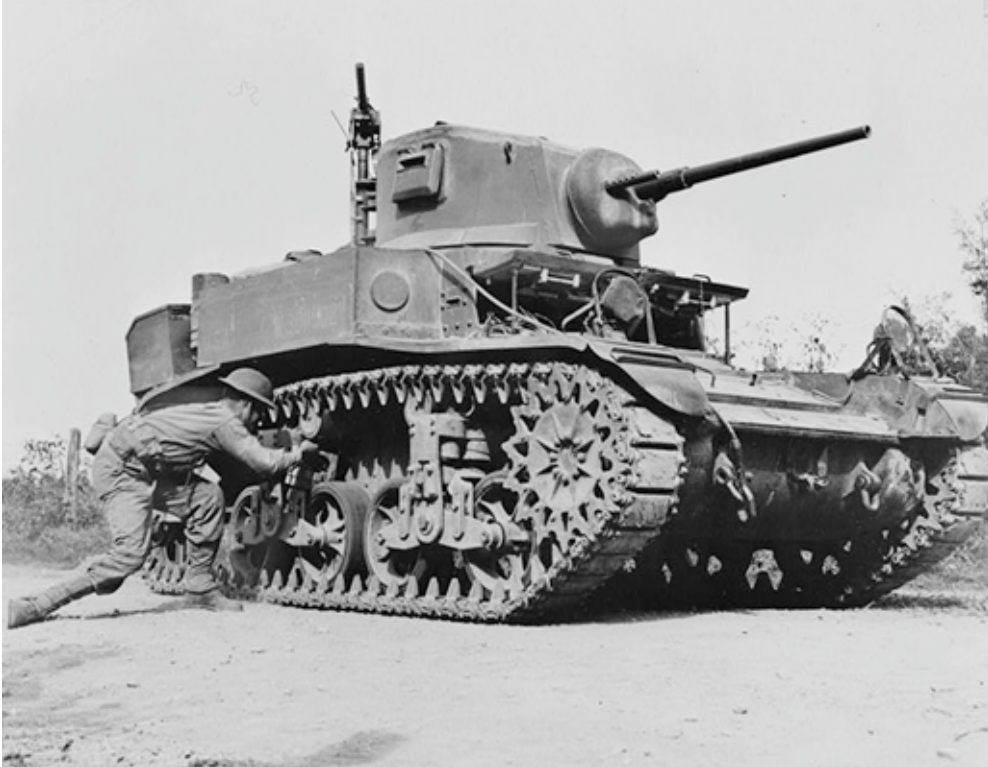
8e00123v: This late-production M3A1 has a welded hull. Note the absence of the sponson machine guns and turret cupola. (Library of Congress, Prints & Photographs Division, FSA-OWI Collection)
