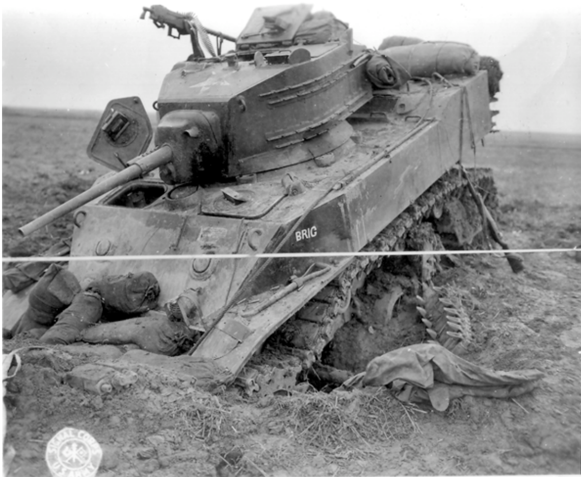
SC-197040: A look at the upper surfaces of the M5A1, courtesy of a German antitank mine. Note the improved hatch arrangement in the extended turret. The white line is tape marking the mined area.
