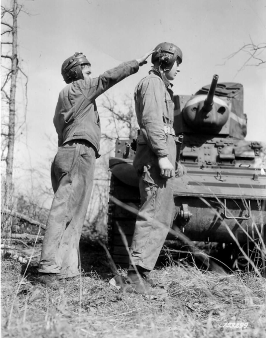
SC-133299: A tank driver learns touch signals that the vehicle commander will use to pass commands to him in his mid-production M3, which has no intercom for the crew. The commander used his foot when in the tank. The direct-vision slits in the front hatches now have armored covers (open here), and the "protectoscope" housing is slightly higher and out-board of that. (NARA, Signal Corps photo)
