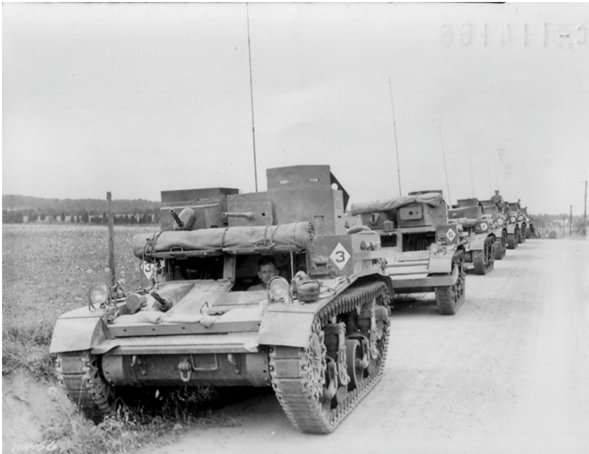
SC-114166: The M2A3 had slightly thicker armor than the M1 combat car and split its upper machine guns between two turrets so that gunners could engage more targets simultaneously. These belong to the 66th Infantry Regiment (Tanks). (NARA, Signal Corps photo)
