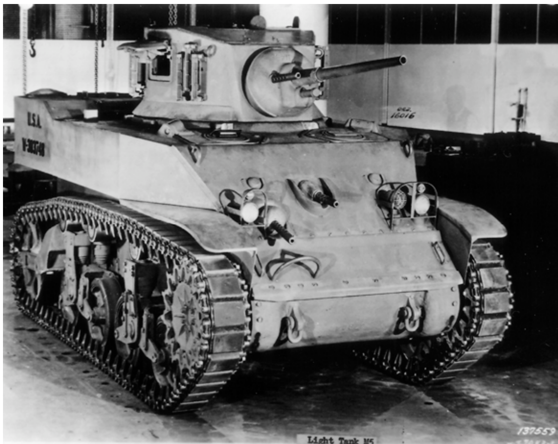
SC-137559-R: The pilot version of the M5 (M3 Experimental) had a fixed hull-mounted machine gun in addition to the one in the ball mount. The sloped front armor provided better protection than the slab-fronted M3, and the hull crew enjoyed overhead hatches with rotating periscopes. (NARA, Signal Corps photo)
