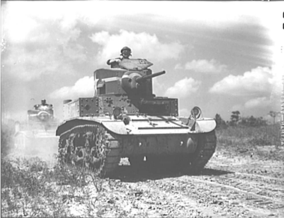
8b04121u: This is an early production M3 Stuart with a welded seven-sided turret and direct vision slits in the front hatches. The hull and sponson machine guns have been temporarily removed. (Library of Congress, Prints & Photographs Division, FSA-OWI Collection)
