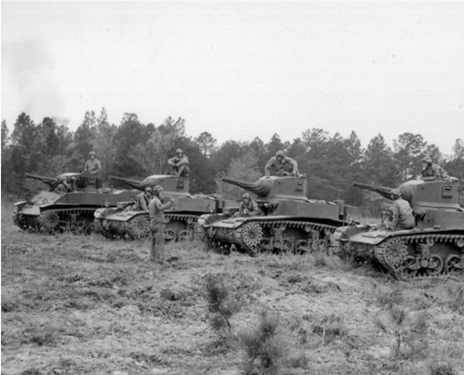
SC-173963: A comparison of the new M5 (left) and several M3A1s with welded hulls. (NARA, Signal Corps photo)
