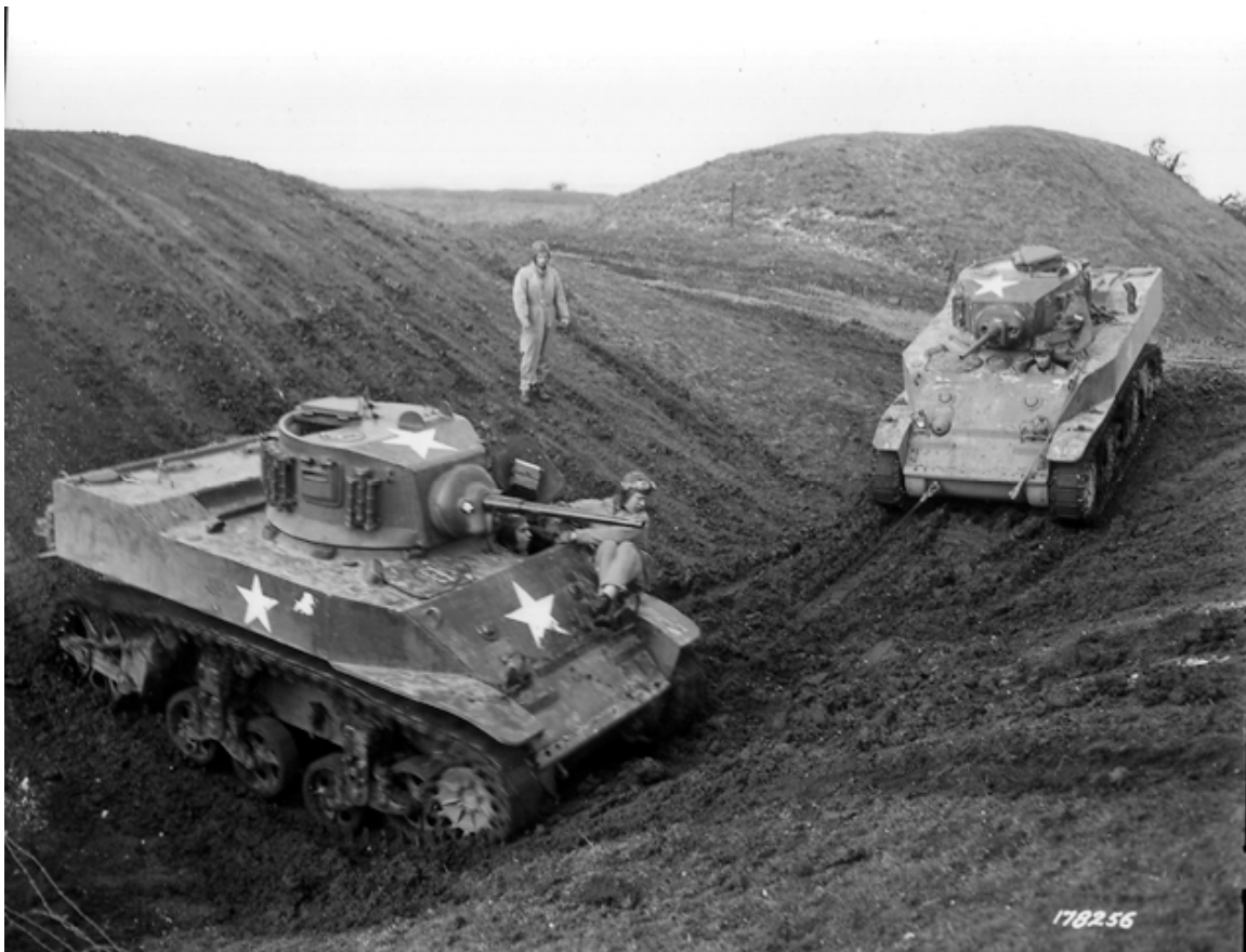
SC-178256: A look at the deck of the M5. These tanks have a triangular commander's hatch, which proved a difficult squeeze for any large man. (NARA, Signal Corps photo)
