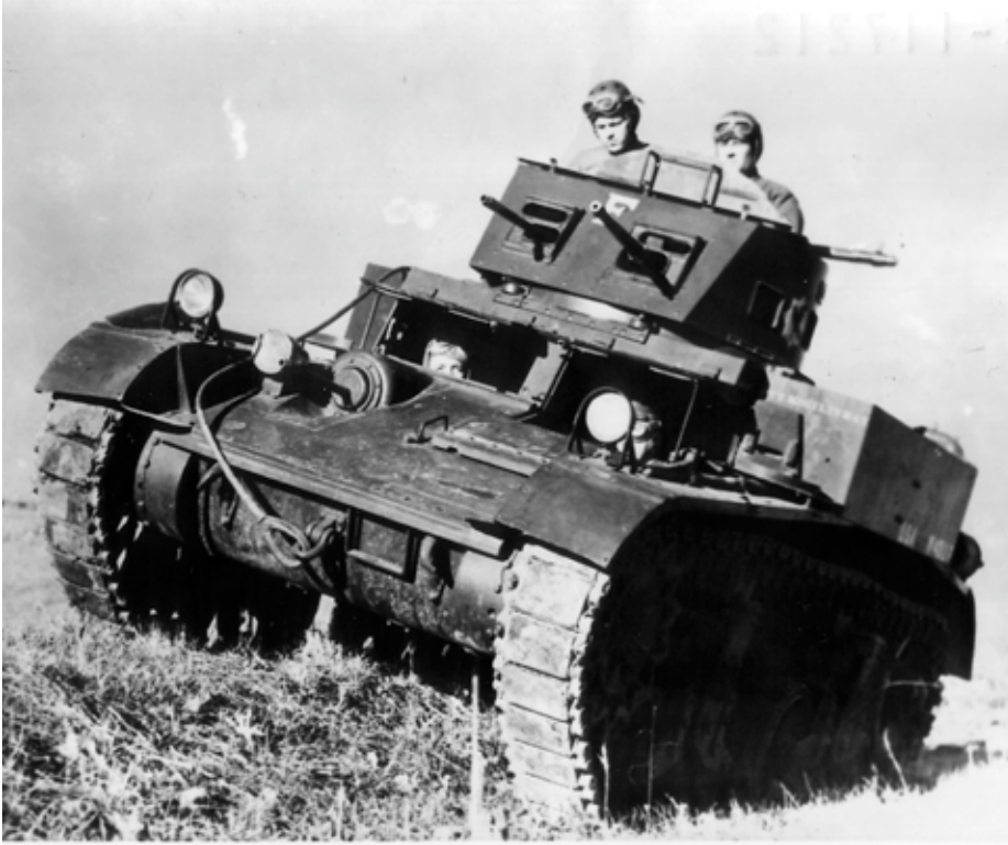
SC-117212: The Combat Car M1/Light Tank M1A2 weighed nearly ten tons and carried one .50-caliber and one .30-caliber machine gun in the turret, plus a .30-caliber in the hull. (NARA, Signal Corps photo)
