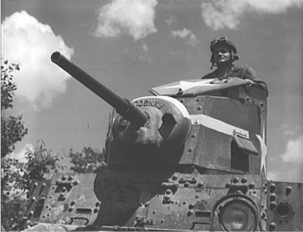
8b04114u: A closer look at the early pattern front hatches with vision slits and the welded seven-sided turret. The turret pistol ports (open here) also had vision slits. (Library of Congress, Prints & Photographs Division, FSA-OWI Collection)
