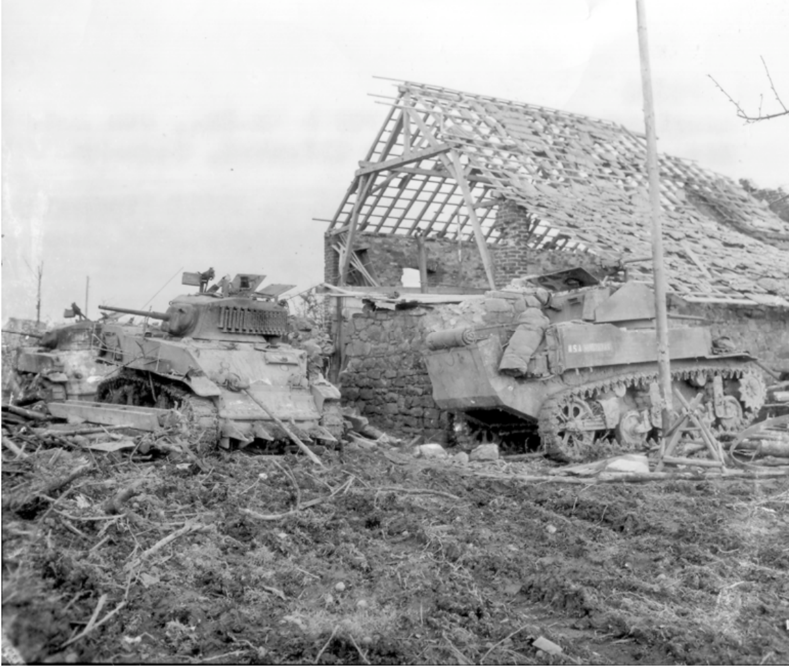
SC-198206: Dog Company, 709th Tank Battalion, light tanks in Kleinhau, Germany. A late-production M5A1, recognizable by a shield covering the machine gun mount on the right turret side, is to the right; it still carries the lower wading kit assembly fitted before it crossed a beach in Normandy. The M5A1 in the center is equipped with a Culin hedgerow device, another Normandy souvenir. (NARA, Signal Corps photo)
