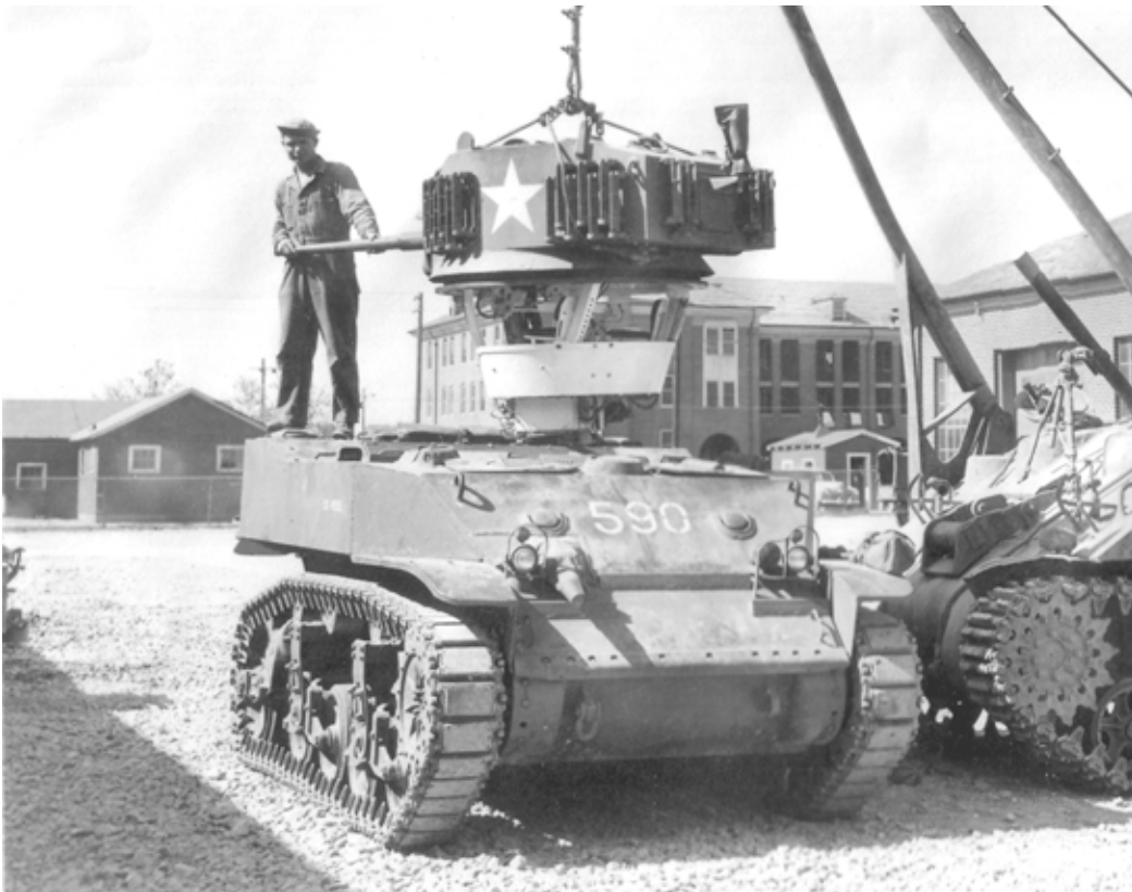
AFB5719: The turret basket on an M5A1; the basket on the M3A1 and M5 looked about the same. (NARA, records of the Chief of Ordnance)
