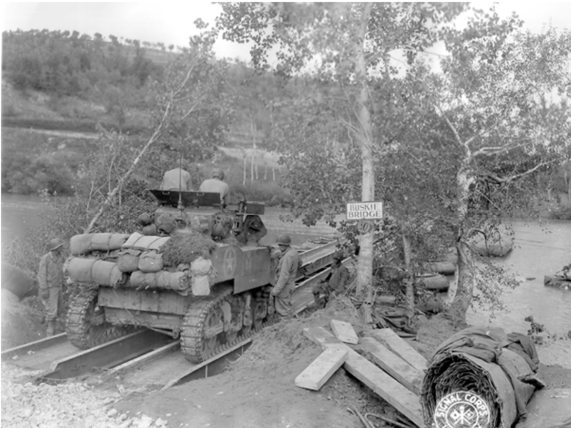
SC-181336: A rear view of an M5A1 laden with the usual bedrolls and other personnel crew gear. This is the first tank to cross the Volturno River via "Huskie Bridge" on 13 October 1944. (NARA, Signal Corps photo)
