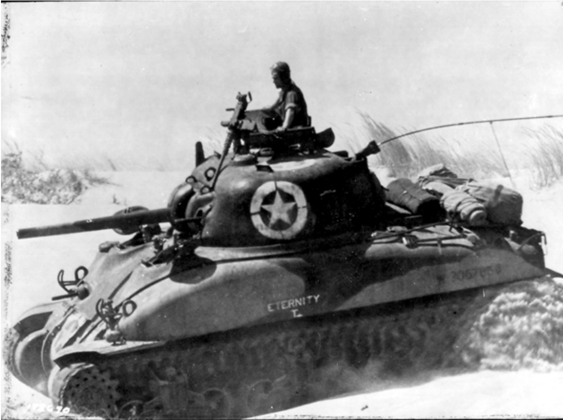
SC-175690: An early production M4A1—almost certainly from the 753d Tank Battalion—plows its way up a Sicilian beach on D-day, 10 July 1943, just after leaving an LCT. The tank has a riveted three-piece final drive housing, the narrow main gun mantlet and simple slit for the coaxial machine gun, and M3 Lee-pattern bogies with the return rollers directly over the center of the assemblies. The driver and bog, however, have fixed periscopes in front of their hatches rather than the very early vision blocks. (NARA, Signal Corps photo)
