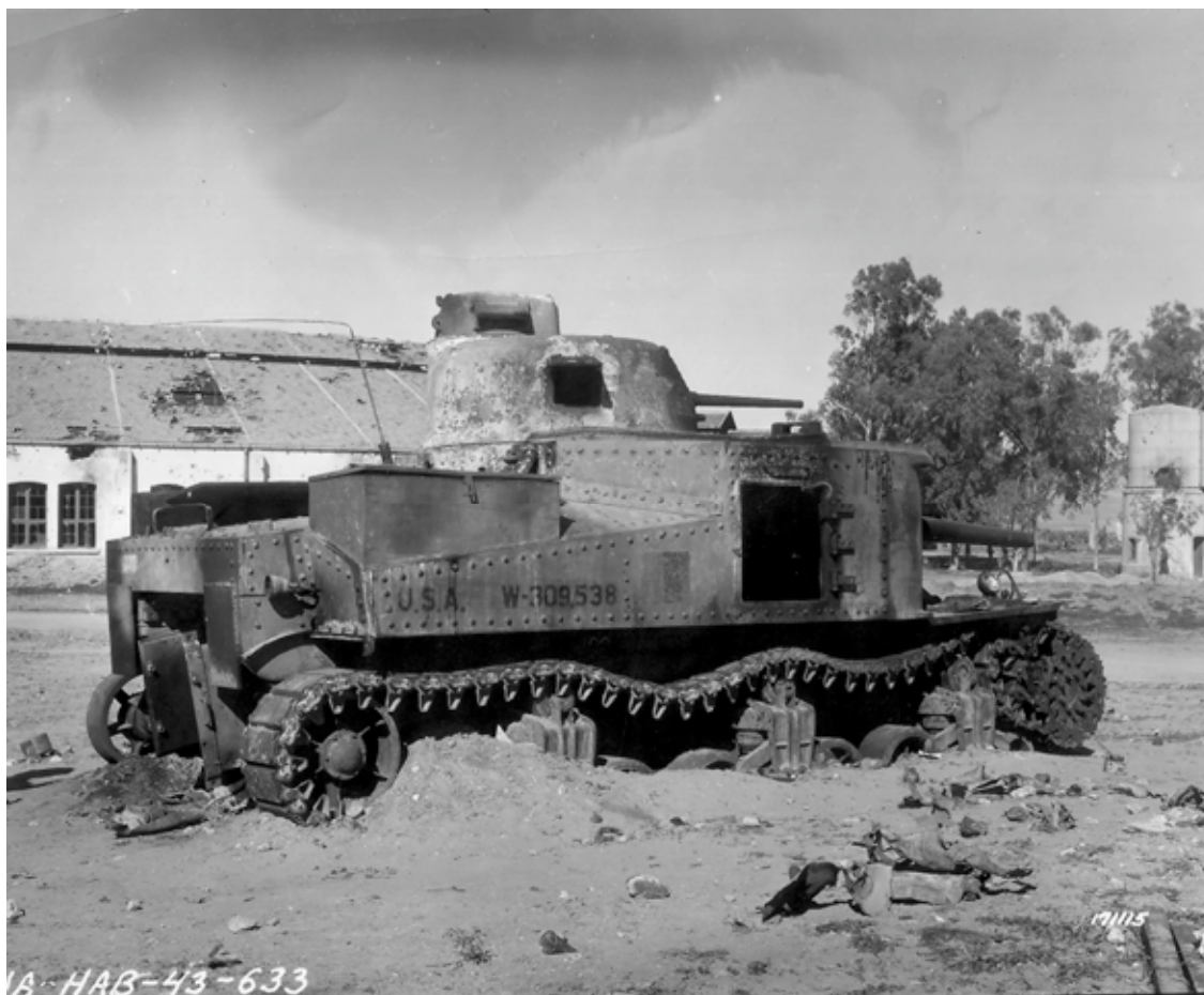
SC-171115: Results of an 88mm gun hit on an M3 Lee. (NARA, Signal Corps photo)
