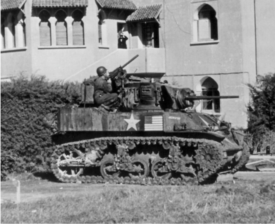
SC-172606: A 70th Tank Battalion M5 crewmember mans the anti-aircraft .30-caliber at Casablanca Airport in November 1942. The new M5 had sloped armor that offered better ballistic protection and twin Cadillac engines, but it retained the M3 Stuart's 37mm main gun. (NARA, Signal Corps photo)
