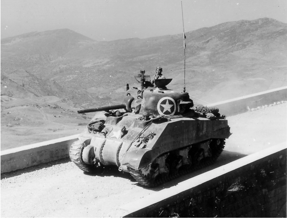
SC-188762: An M4 near Mistretta, Sicily, in August 1944 provides a view of the hatch arrangements and the armored cover added to protect the slit through which the coaxial machine gun protrudes. Terrain such as this constricted tank operations. (NARA, Signal Corps photo)
