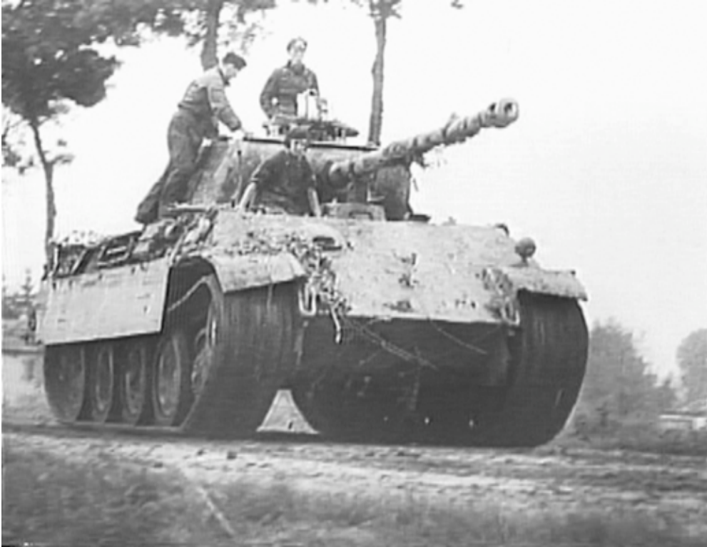
242-MID-3425_2: A Panther rolls toward Luneville during the counterattack against Patton's Third Army in Lorraine. The Mark V outclassed even late-production Shermans in fire power and armor, but it was mechanically less reliable, weighed half again as much, and consumed more fuel. (National Archives, German newsreel)
