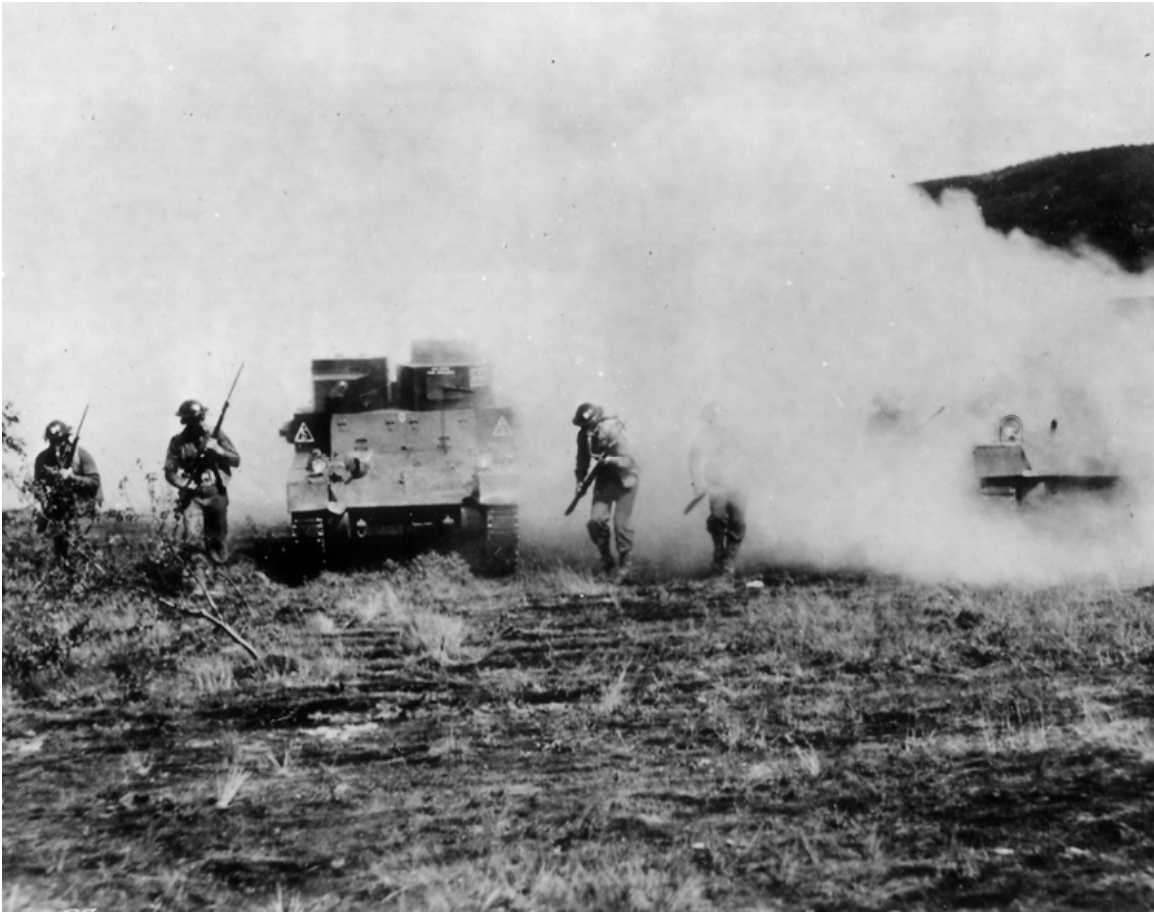
SC-114197: One view of tanks emphasized their infantry-support role dating back to World War I. Here, M2A3 light tanks from the 66th Infantry Regiment (Tanks) and foot troops attack through a smoke screen during maneuvers in August 1939. (NARA, Signal Corps photo)
