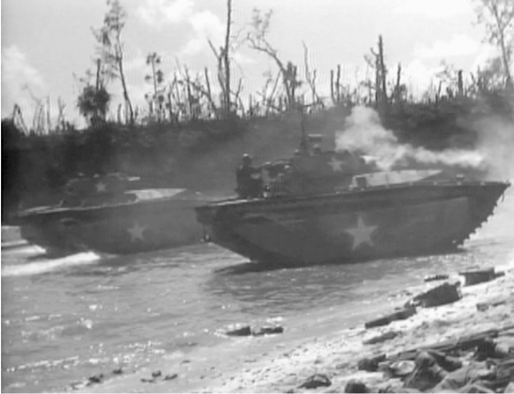
111-ADC-2460_3: A 776th Amphibian Tank Battalion LVT(A)(4) supporting the 81st Infantry Division's landings on 17 September 1944 at Angaur, Pelau Islands, fires its 75mm main gun at Japanese troops from the waterline. Only one battalion man was killed that day. (U.S. Navy film)
