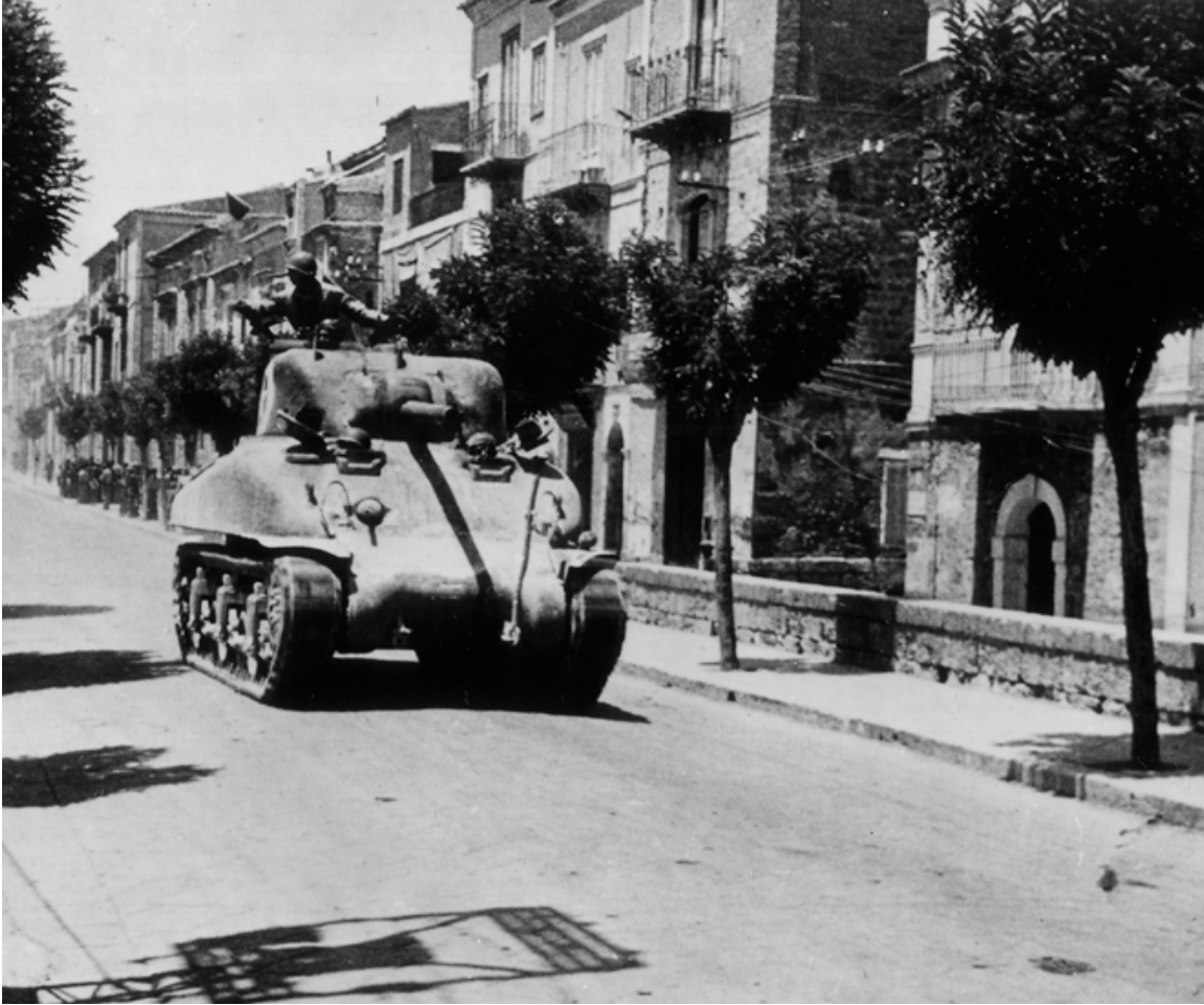
SC-180520: A CCB/2d Armored Division M4A1 drives through Gela, Sicily, on 11 July 1943. This vehicle has the early pattern bogies and is equipped with direct vision blocks. It is nonetheless outfitted with the second-generation cast final drive housing. (NARA, Signal Corps photo)
