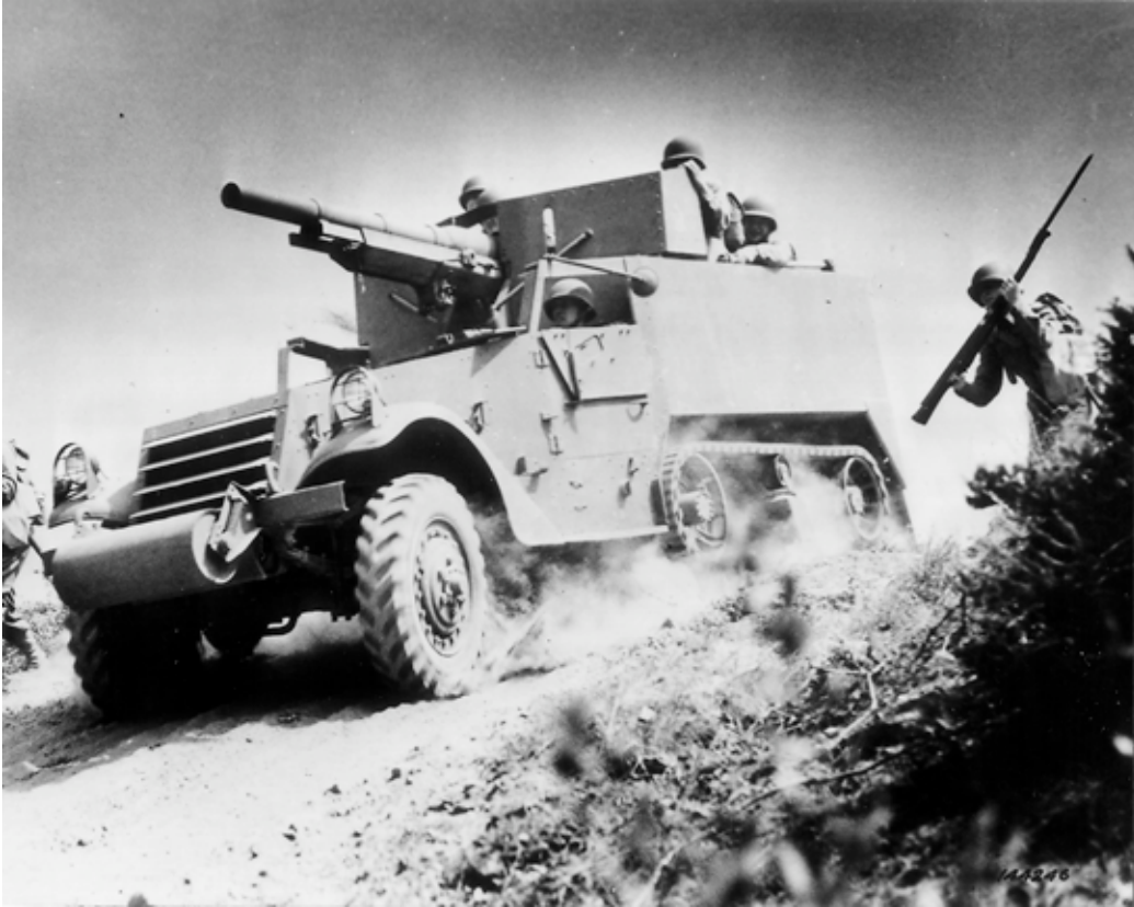
SC-144246: According to U.S. Army doctrine, the tank destroyer—here the stopgap M3 mounting a 75mm gun—was supposed to battle enemy tanks while friendly tanks dealt with other targets. (NARA, Signal Corps photo)
