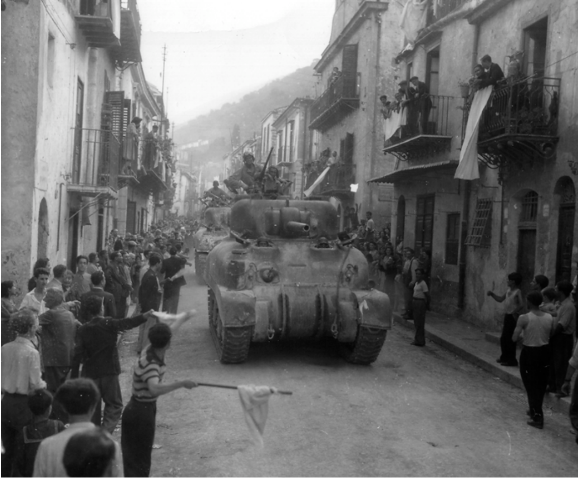
SC-179709: Second Armored Division tanks on 22 July 1943 enter Palermo, Sicily, as residents waive white flags. The lead M4A1 has an add-on armor piece that was often affixed around the coaxial machine gun to prevent shrapnel or bullets from entering the turret. The lead tank has sand shields on the sides. (NARA, Signal Corps photo)
