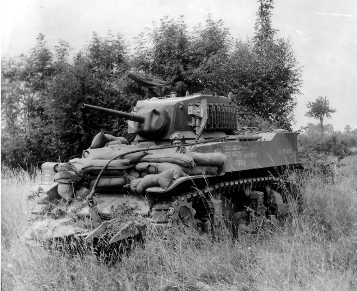
SC-192066: Tank battalions adopted new techniques in the hedgerows. A 709th Tank Battalion M5A1 in July 1944 has sandbags for extra armor protection and the Culin hedgerow-busting device that allowed tanks to plow through the obstructions. (NARA, Signal Corps photo)
