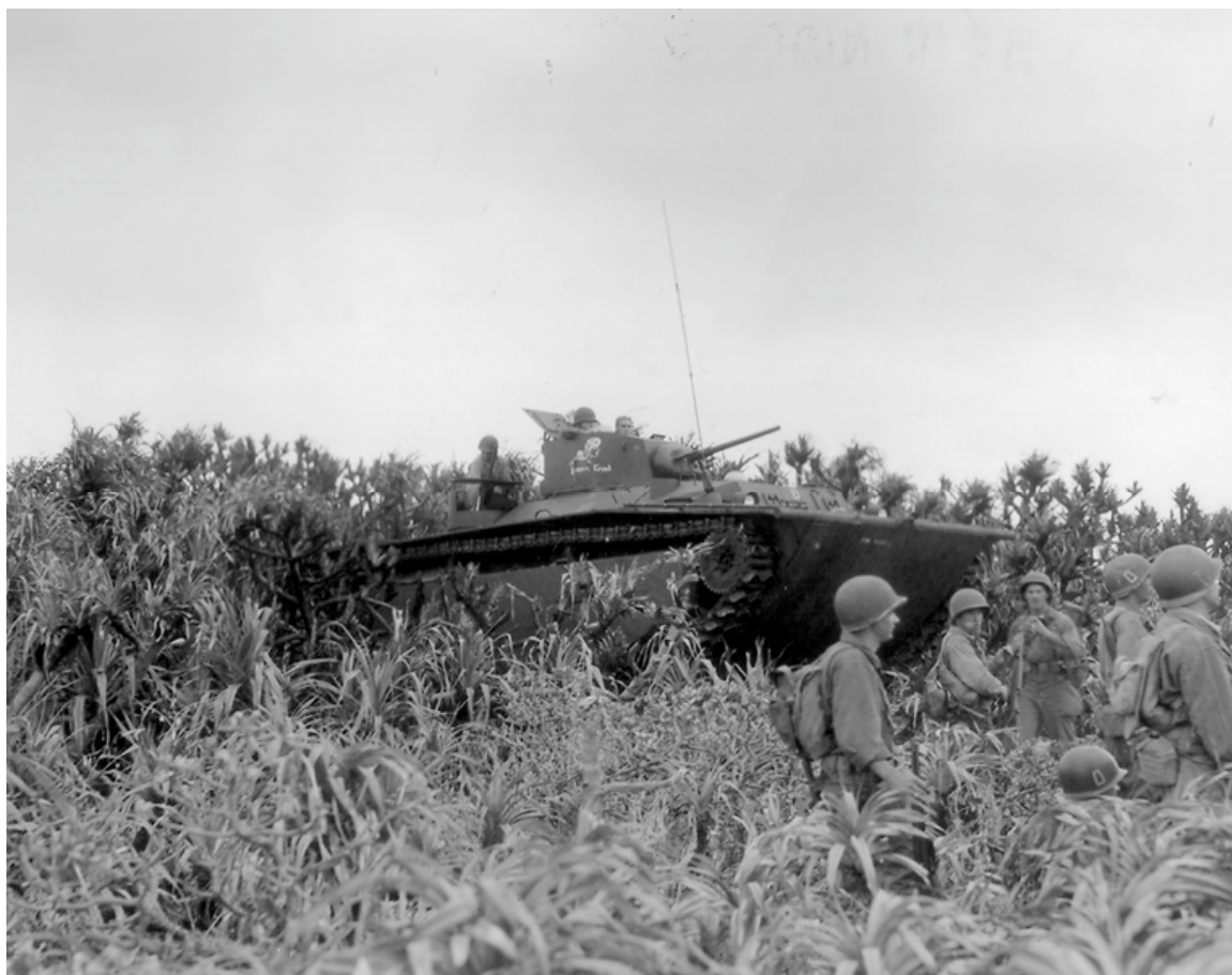
SC-206493: A 708th Amphibian Tank Battalion LVT(A)(1), which was the first type of amtank produced, works inland with the 77th Infantry Division on Keise Shima on 31 March 1945. (NARA, Signal Corps photo)
