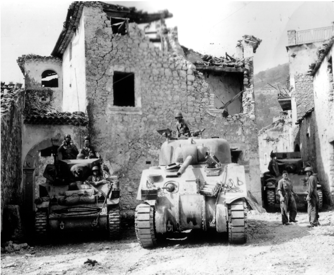
SC-190082: 755th Tank Battalion medium and light tanks in Coreno, Italy, just after its capture on 14 May 1944. The M4 exhibits first-generation characteristics in nearly every respect, although it has appliqué armor over the gunner's position. (NARA, Signal Corps photo)
