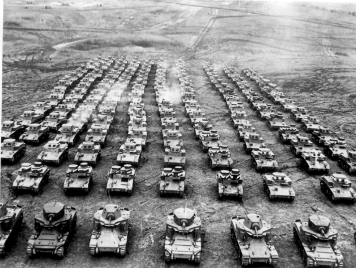
SC-118008: Part of the 1st Armored Division's tank brigade in formation at Fort Knox in March 1941. The tanks are a hodgepodge of prewar models. M2 and M2A1 medium tanks, the latter with larger turrets, form the front line. They carry a 37mm main gun and bristle with machine guns. The rest are light tanks and combat cars, the most modern being the M2 light tank with a 37mm gun. (NARA, Signal Corps photo)
