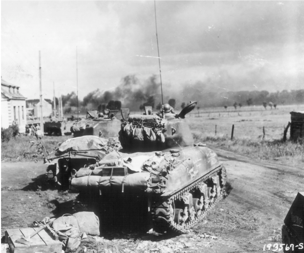
SC-193567-S: Tanks blast German infantry near Gelim, Belgium, on 3 September 1944 as Allied forces drive toward the western border of the Reich and its Siegfried Line. The tank to the right is an M4A1 (76mm), which provided the commander with a vision cupola and single-piece hatch. The tanks' rubber chevron tracks show the heavy wear inflicted by the long race from Normandy. An M4 with its split commander's hatch and with rubber block tracks is to the left. (NARA, Signal Corps photo)
