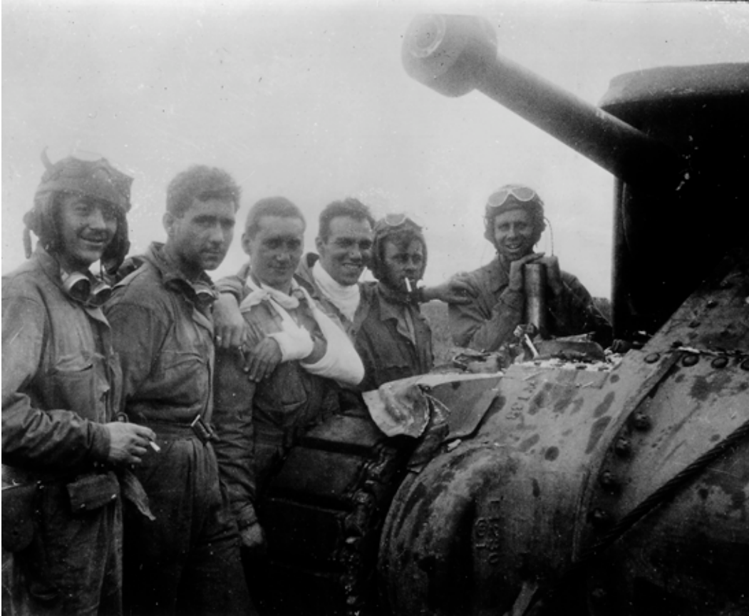
SC-149998: A 1st Armored Division M3 Lee tank crew (2/13th Armored Regiment) poses after the capture of Oran in November 1942. Both men and tank look like they are now veterans. The 75mm gun is in a limited traverse side sponson; this one is a short-barreled M2 version weighted to work with a retrofitted gyro stabilizer. (NARA, Signal Corps photo)
